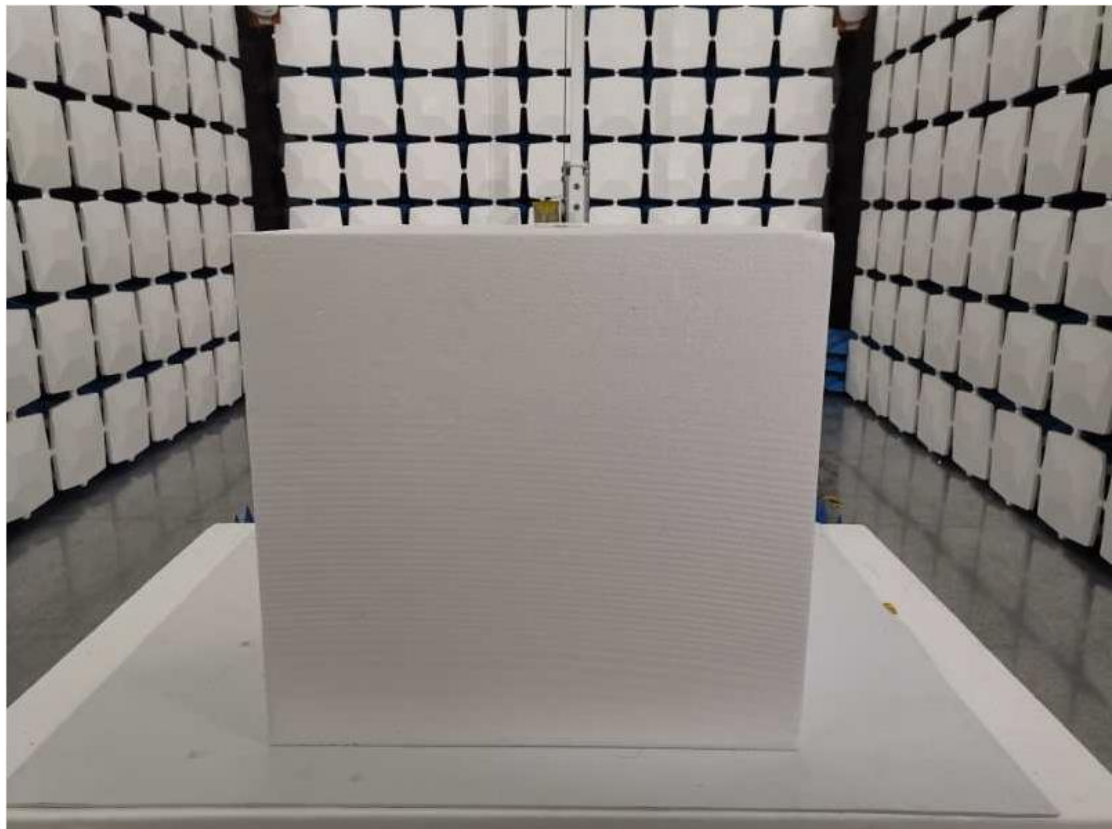
Above 1GHz for radiated emission test setup
