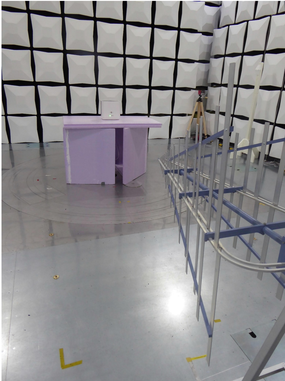
Test setup semi-anechoic chamber M276, 30 MHz - 1 GHz
