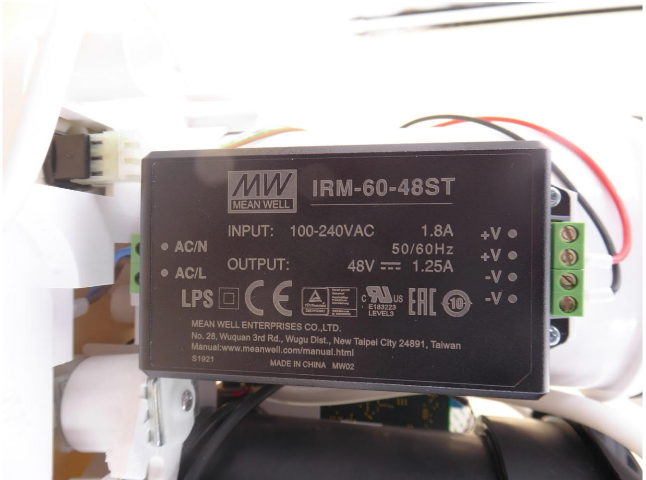
AC/DC converter, detail view
