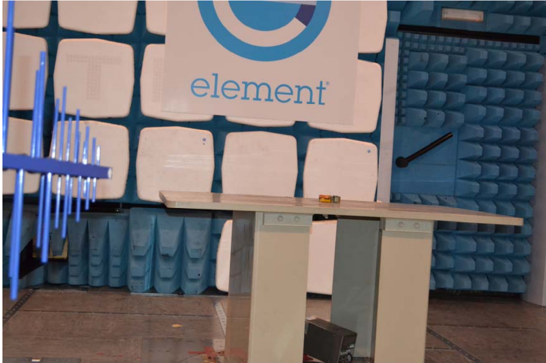
Radiated setup above 1 GHz
