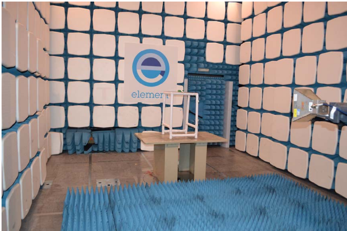
Radiated setup above 1 GHz
