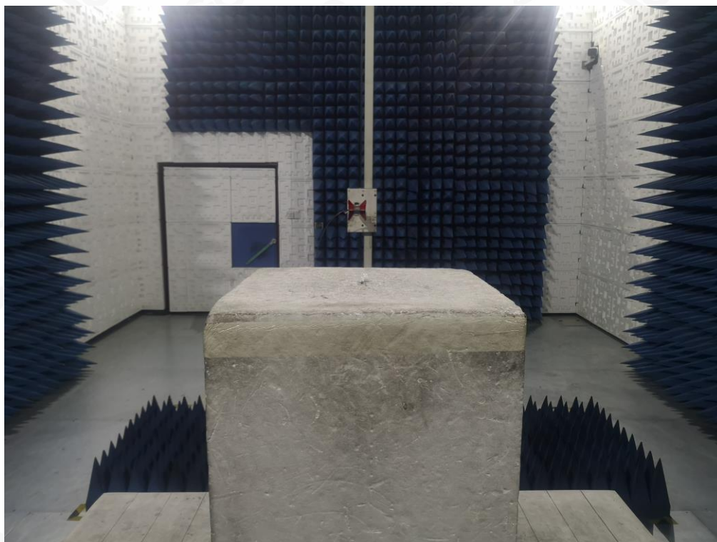
RADIATED EMISSION TEST SETUP ABOVE 1GHZ
