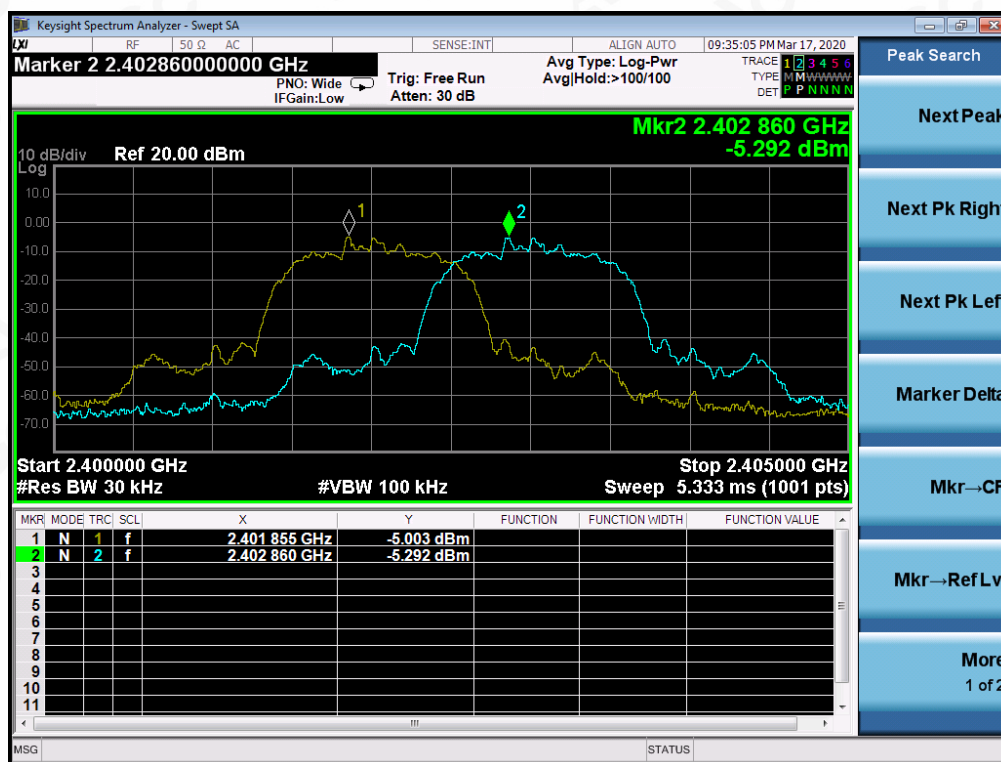
TEST PLOT FOR FREQUENCY SEPARATION
