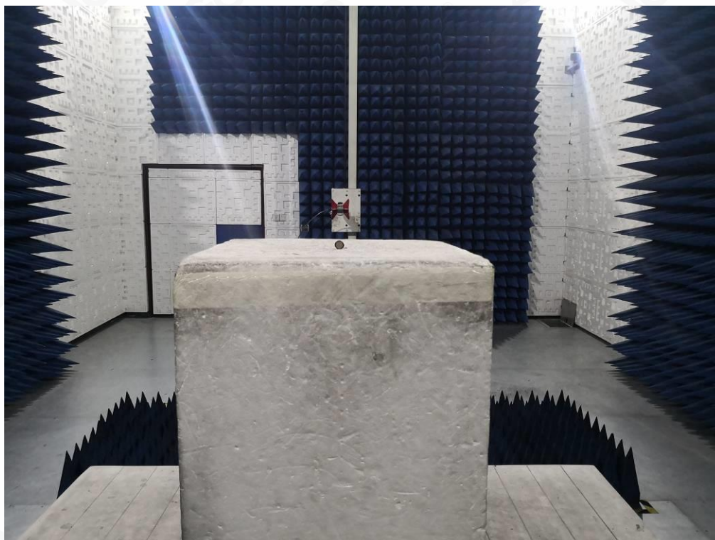
RADIATED EMISSION TEST SETUP ABOVE 1GHZ
