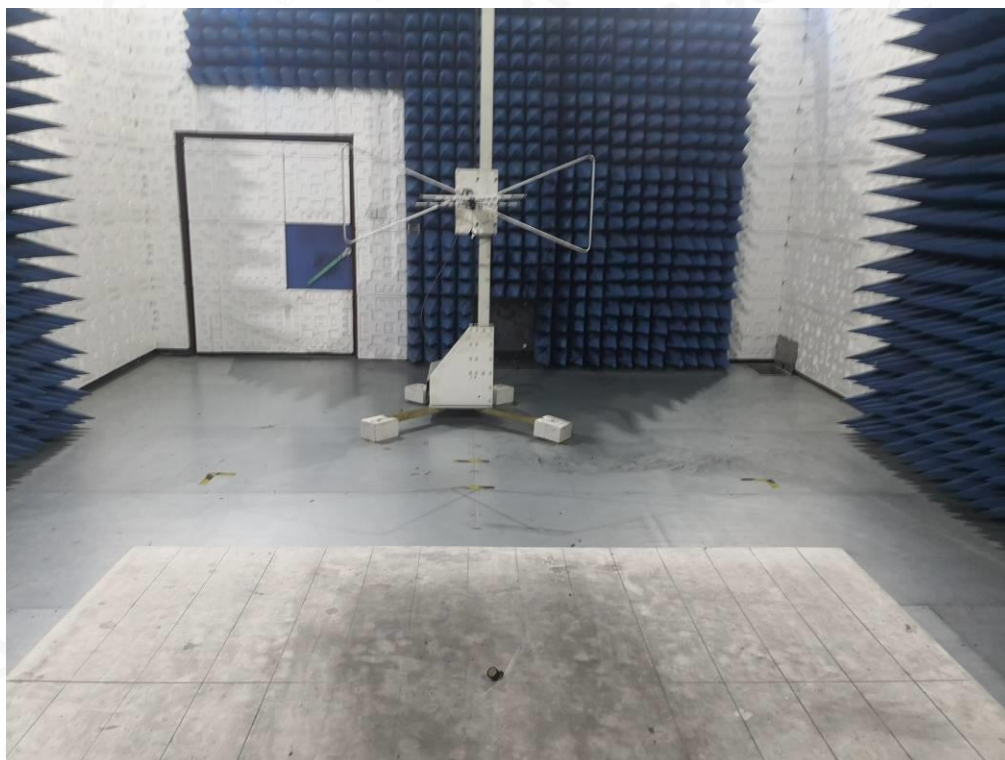
RADIATED EMISSION TEST SETUP ABOVE 1GHZ
