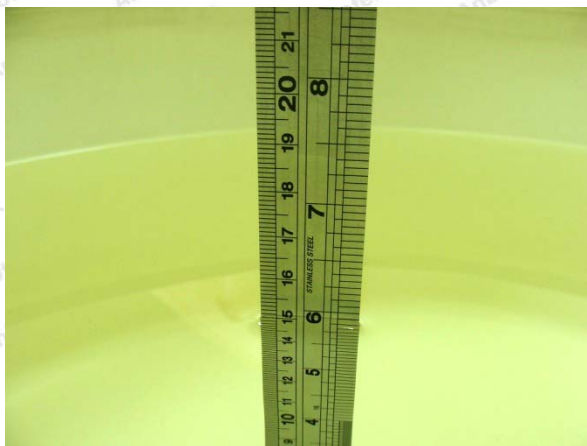
Photo of Liquid Height for Body SAR
