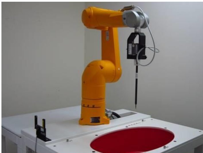
Fig.1 Photograph of the SAR measurement system
