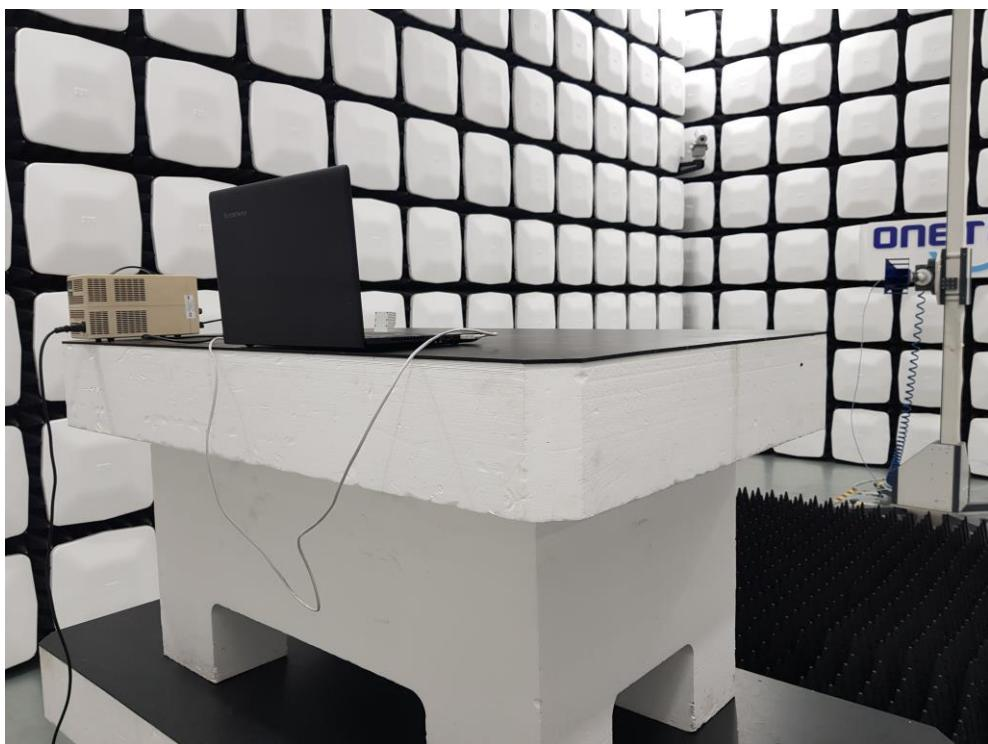
**- Radiated Emission Test (Above 1 GHz) [Adapter]**
