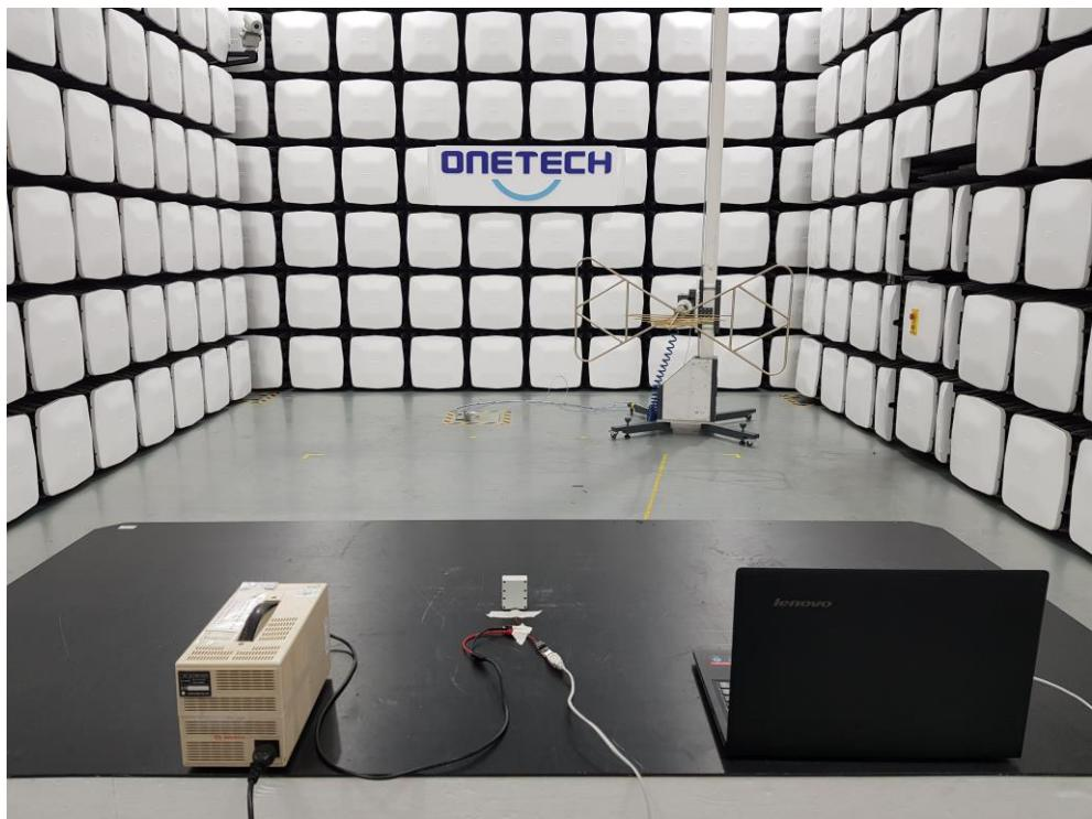
**- Radiated Emission Test (Below 1 GHz) [Adapter]**
