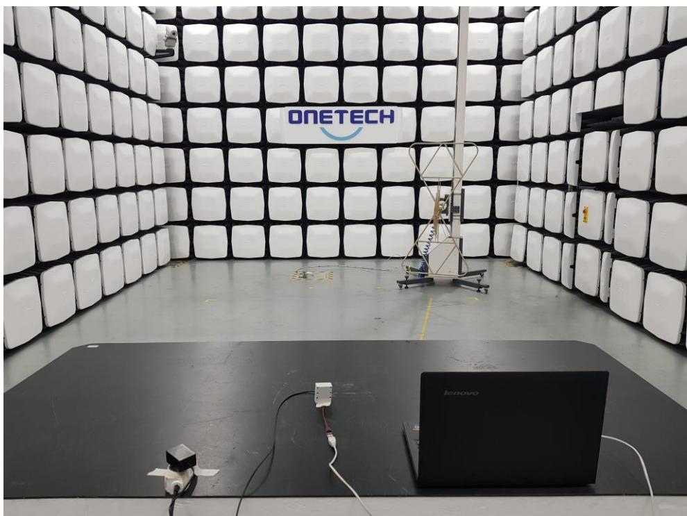
**- Radiated Emission Test (Below 1 GHz) [DC Power]**
