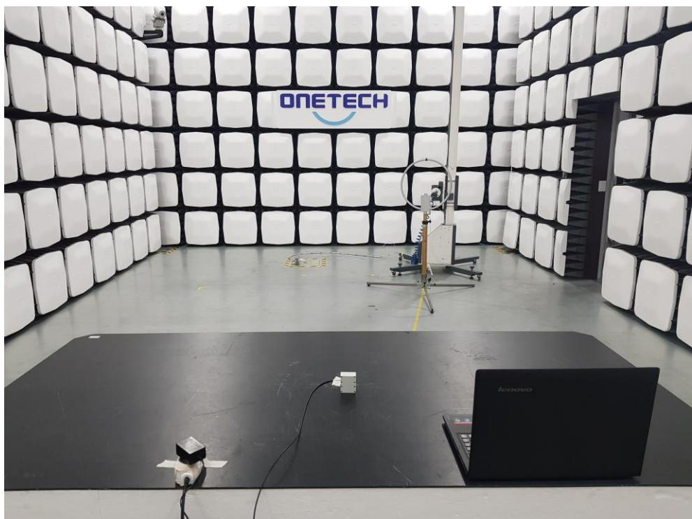
**- Radiated Emission Test (Above 1 GHz) [DC Power]**
