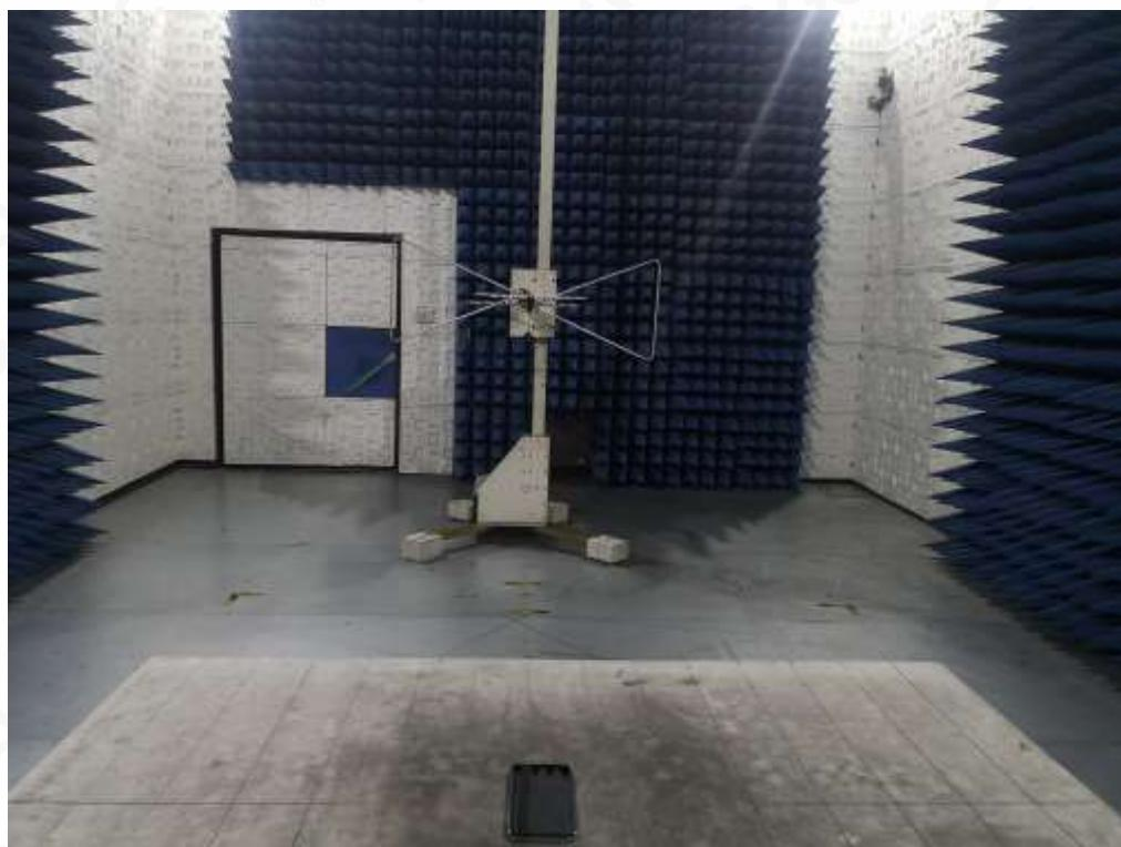
**RADIATED EMISSION TEST SETUP ABOVE 1GHZ**
