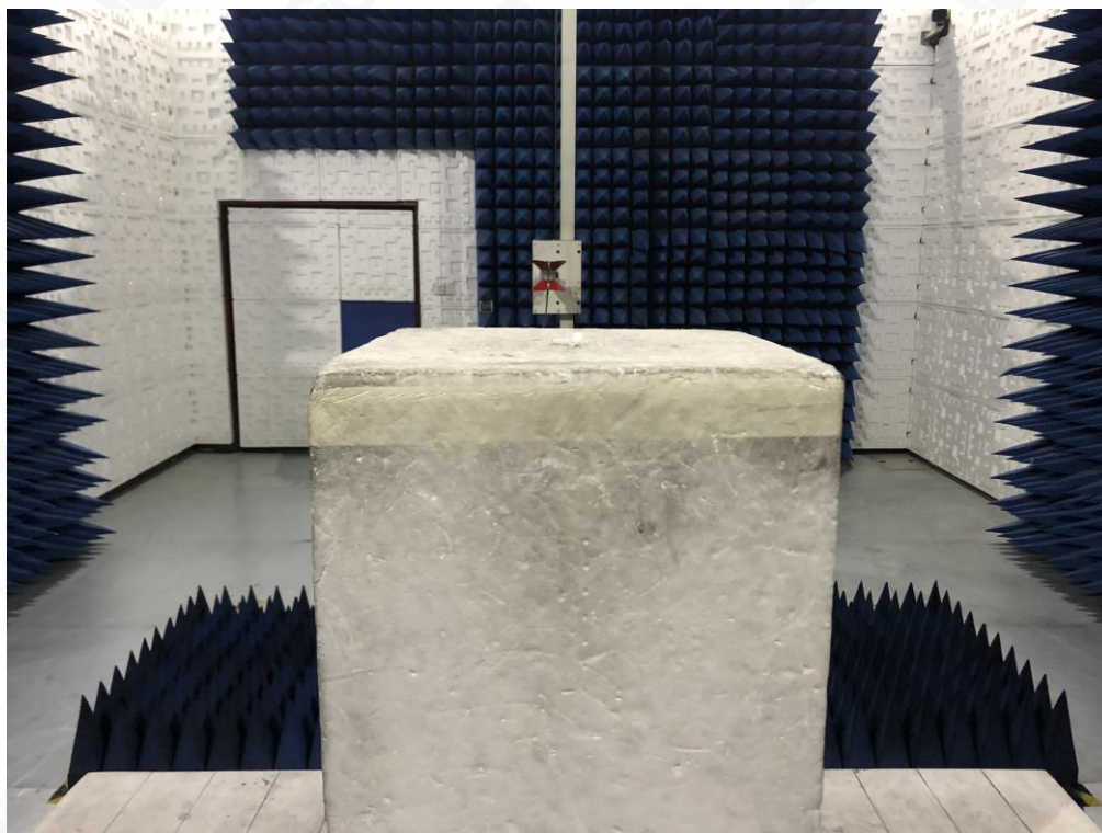
RADIATED EMISSION TEST SETUP ABOVE 1GHZ
