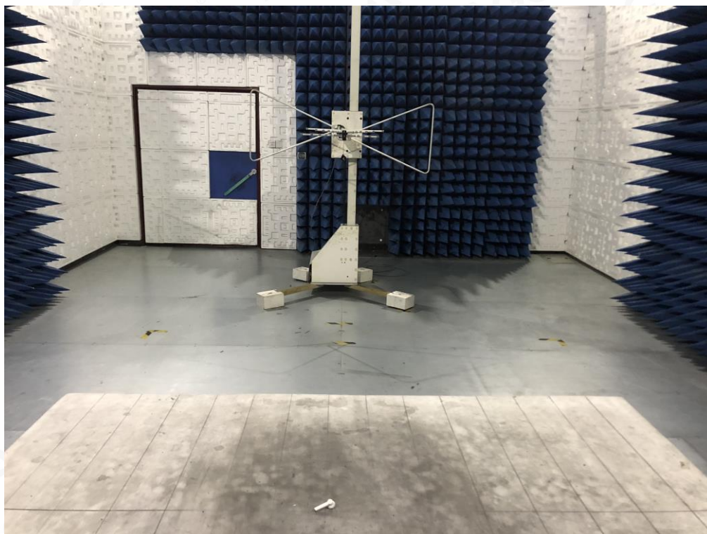
RADIATED EMISSION TEST SETUP ABOVE 1GHZ
