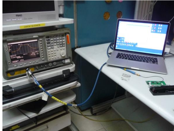
Photograph No.4 Setup for OBW measurements
