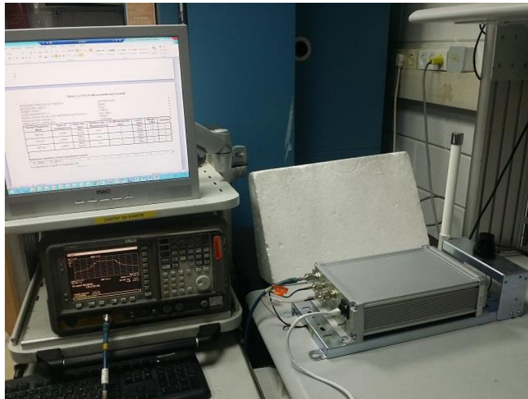
Photograph No.4 Setup for OBW measurements
