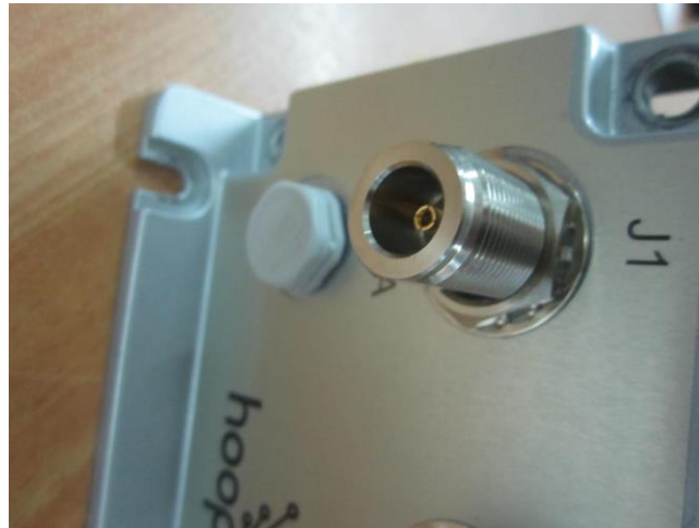
Photograph No.3 Antenna connector
