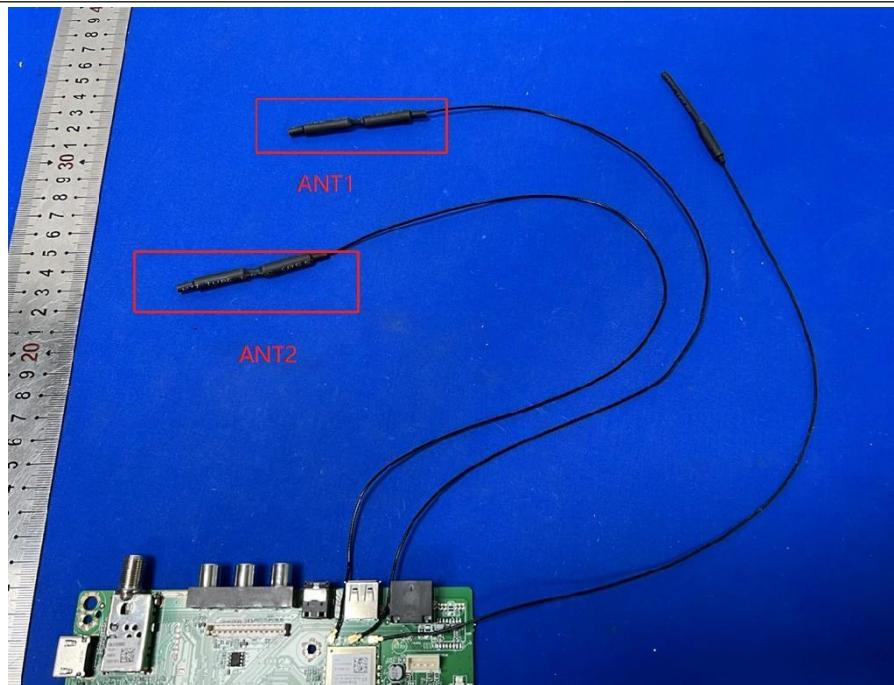
The antenna is Metal antenna.ANT1/ANT2=0.97dBi
