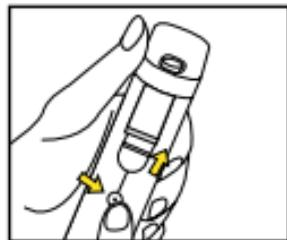
4. Press and hold the power button for 3 seconds to turn on. Slide the built-in cutter upward to cut the label.
