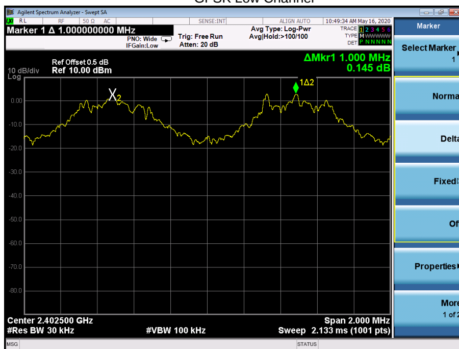
Test plots GFSK Low Channel
