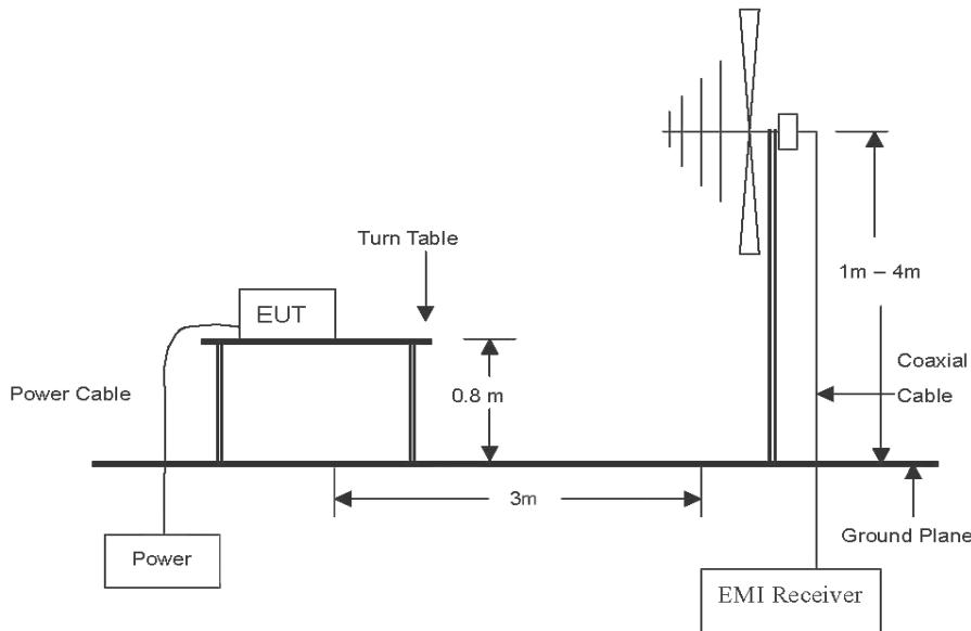
The diagram below shows the test setup that is utilized to make the measurements for emission from 1 GHz to the tenth harmonic of the highest fundamental frequency or to 40 GHz emissions, whichever is lower.
