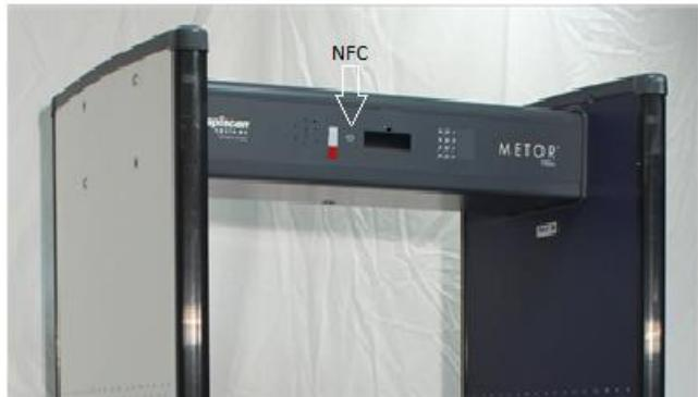
The NFC module is situated at about 214cm (84 inch) height from the ground level and the spiral rectangular antenna is situated parallel to the cross piece surface with maximum field strength perpendicular to the center of the surface.
