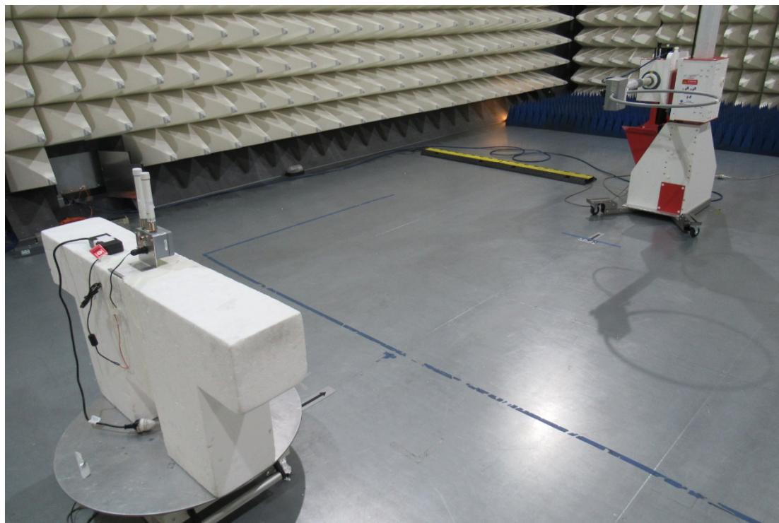
Radiated Emissions: 9 kHz – 30 MHz
