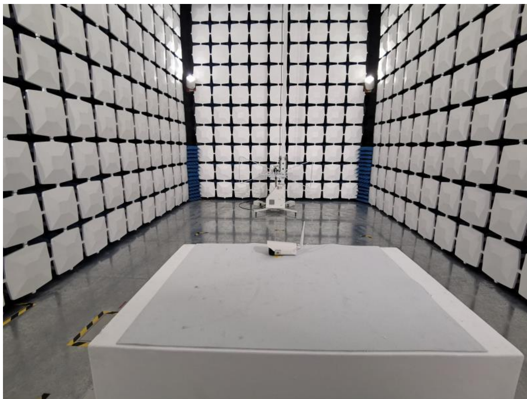
Below 1GHz for radiated emission test setup
