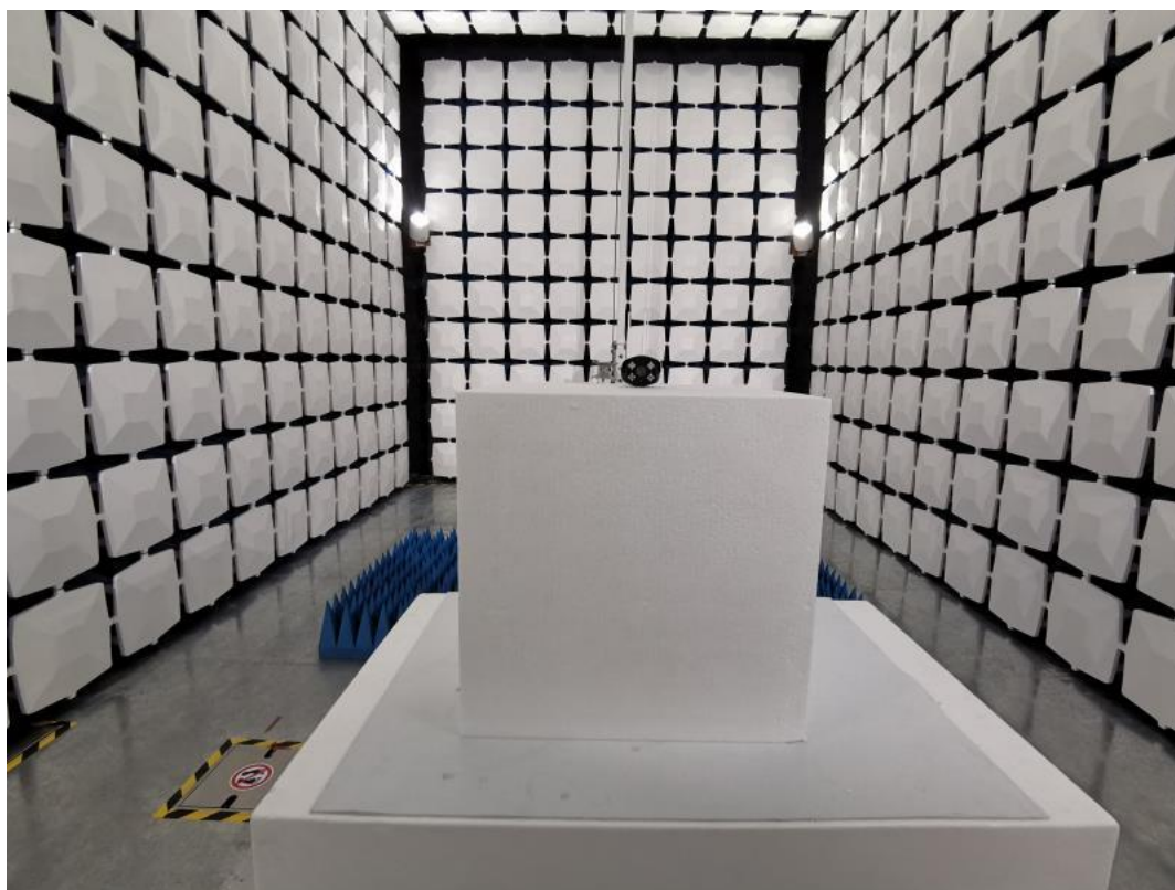
Above 1GHz for radiated emission test setup
