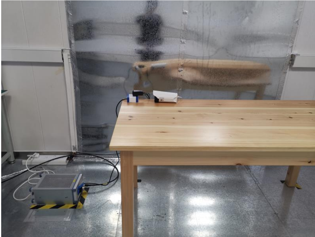
Conducted Emission Test setup
