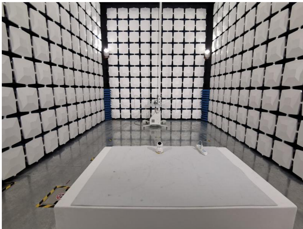
Below 1GHz for radiated emission test setup
