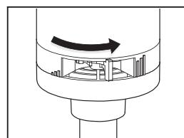
Raise/ Increase the buzzer volume by sliding the control lever to the right as shown in the diagram to the left.
