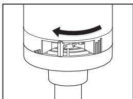
Buzzer volume is reduced by sliding the volume control lever to the left as shown in the diagram to the left.
