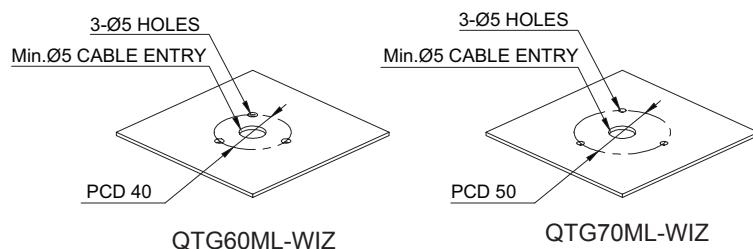
② Remove the flange nuts from bolts and place the product through the mounting surface holes.
