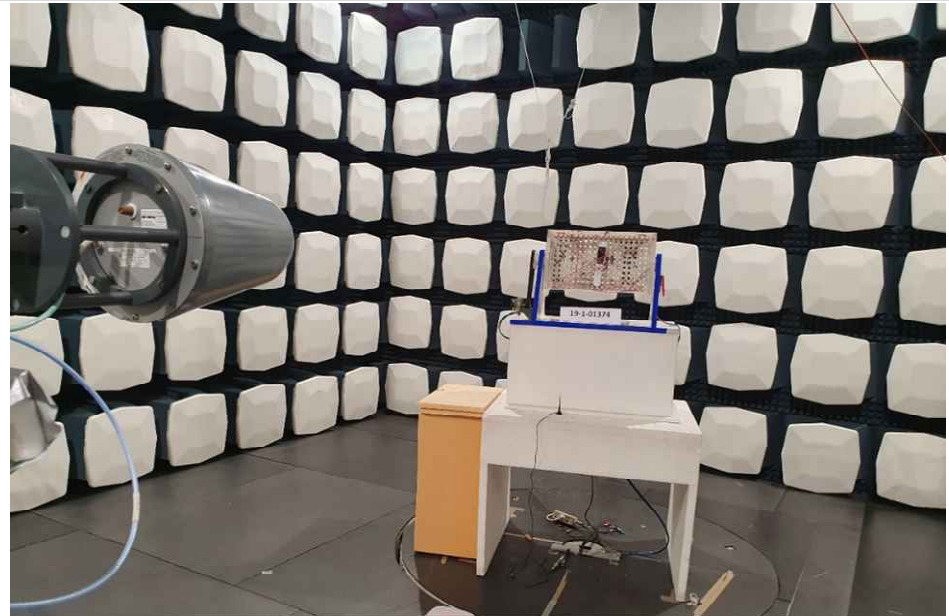
Photograph 5: EUT Test Setup in the fully anechoic chamber, overall view
