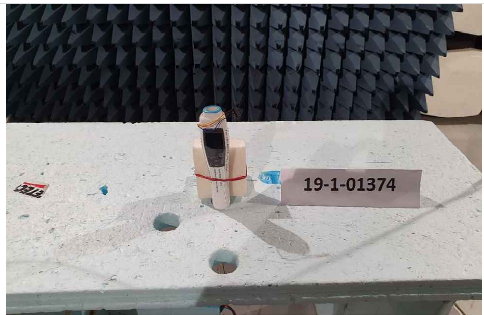
Photograph 2: EUT Test Setup in the semi anechoic chamber, close-up view
