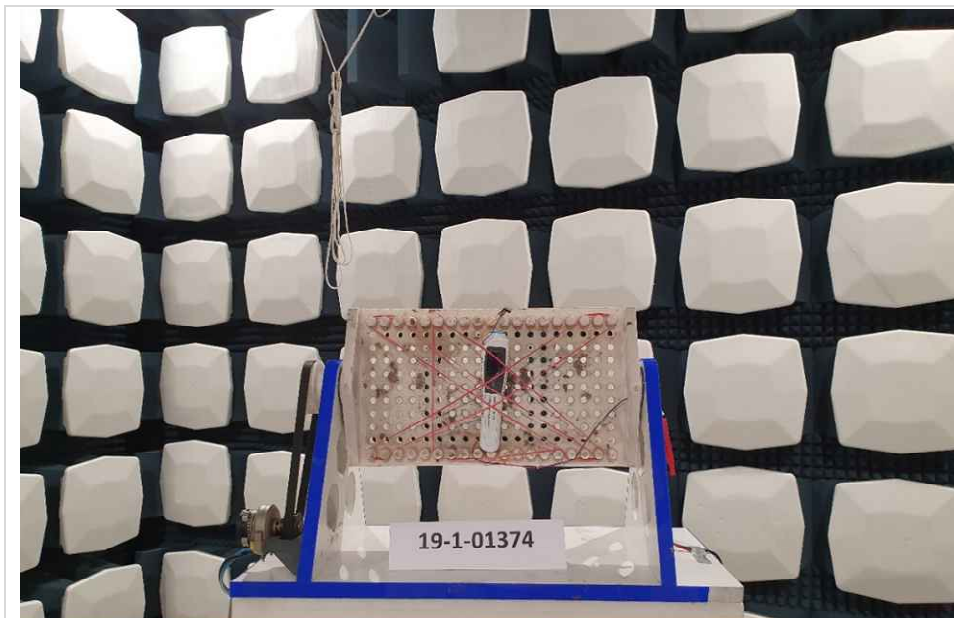
Photograph 6: EUT Test Setup in the fully anechoic chamber, close-up view
