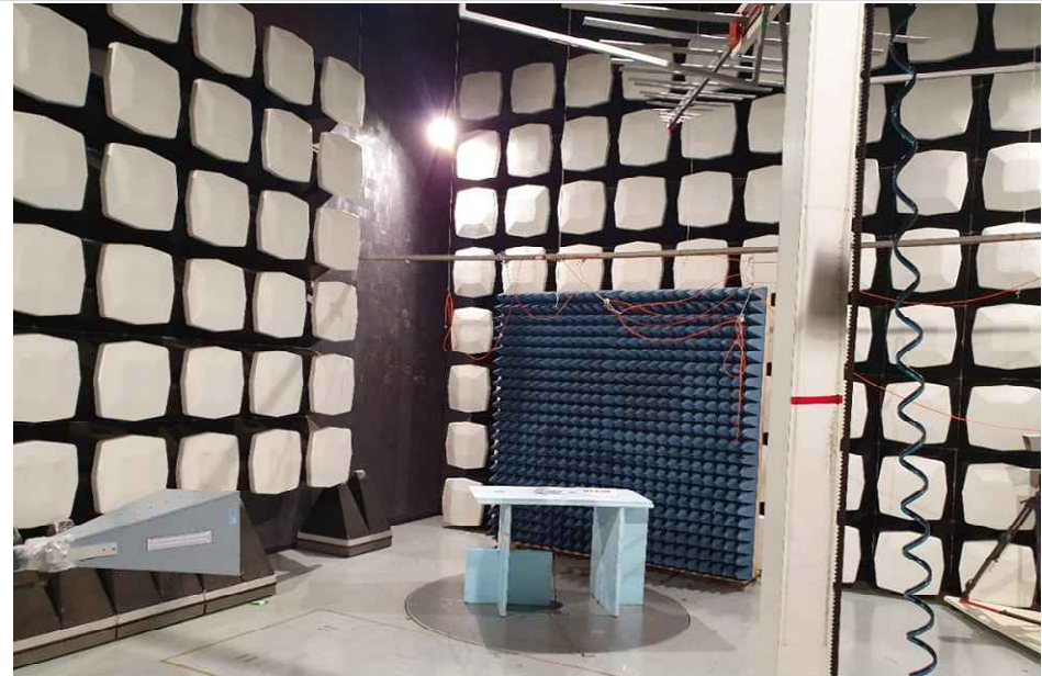
Photograph 3: EUT Test Setup in the semi anechoic chamber, overall view
