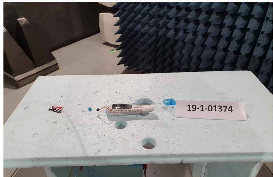
Photograph 4: EUT Test Setup in the semi anechoic chamber, close-up view
