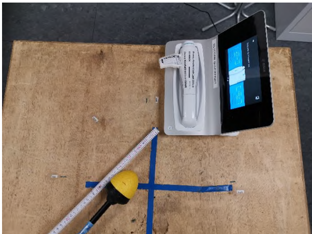
Photograph 5: Setup in the shielded room for E-field strength on position B at a distance of 15 cm
