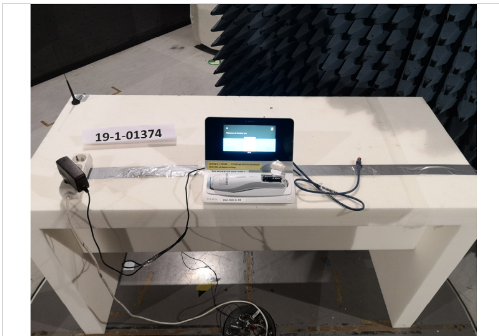
Photograph 10: EUT Setup Magnetic Field Measurements in the Semi anechoic chamber
