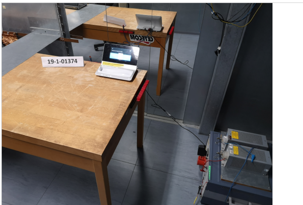
Photograph 6: EUT Setup Conducted emissions on AC-Power lines
