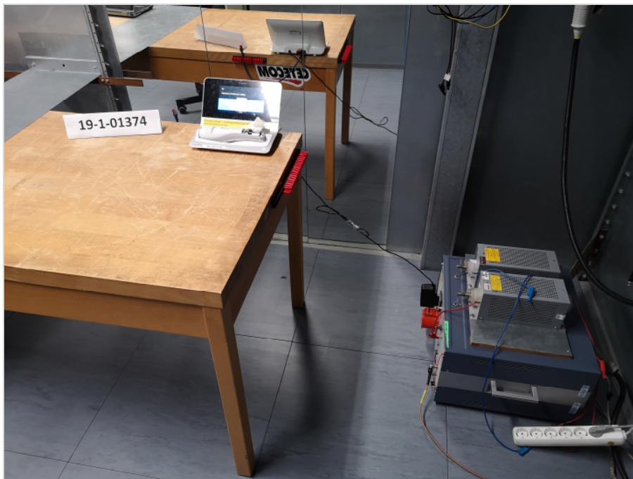
Photograph 12: EUT Setup Conducted emissions on AC-Power lines
