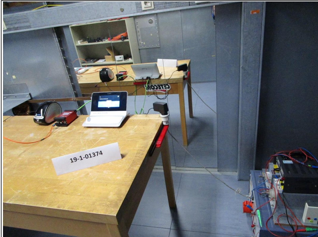
Photograph 1: Conducted measurements test set-up
