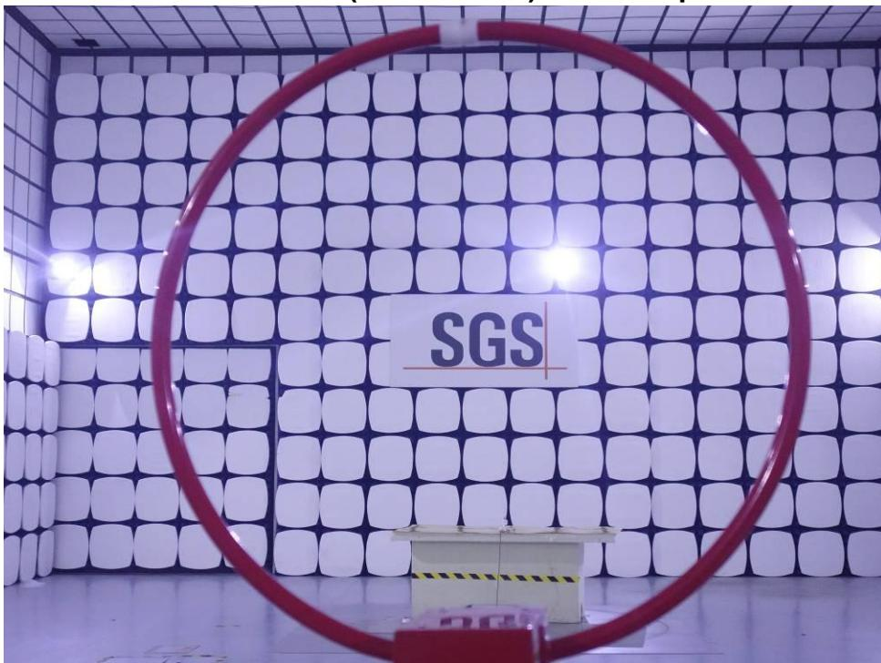
**1.4 Radiated Emissions(30MHz-1GHz) Test Setup**
