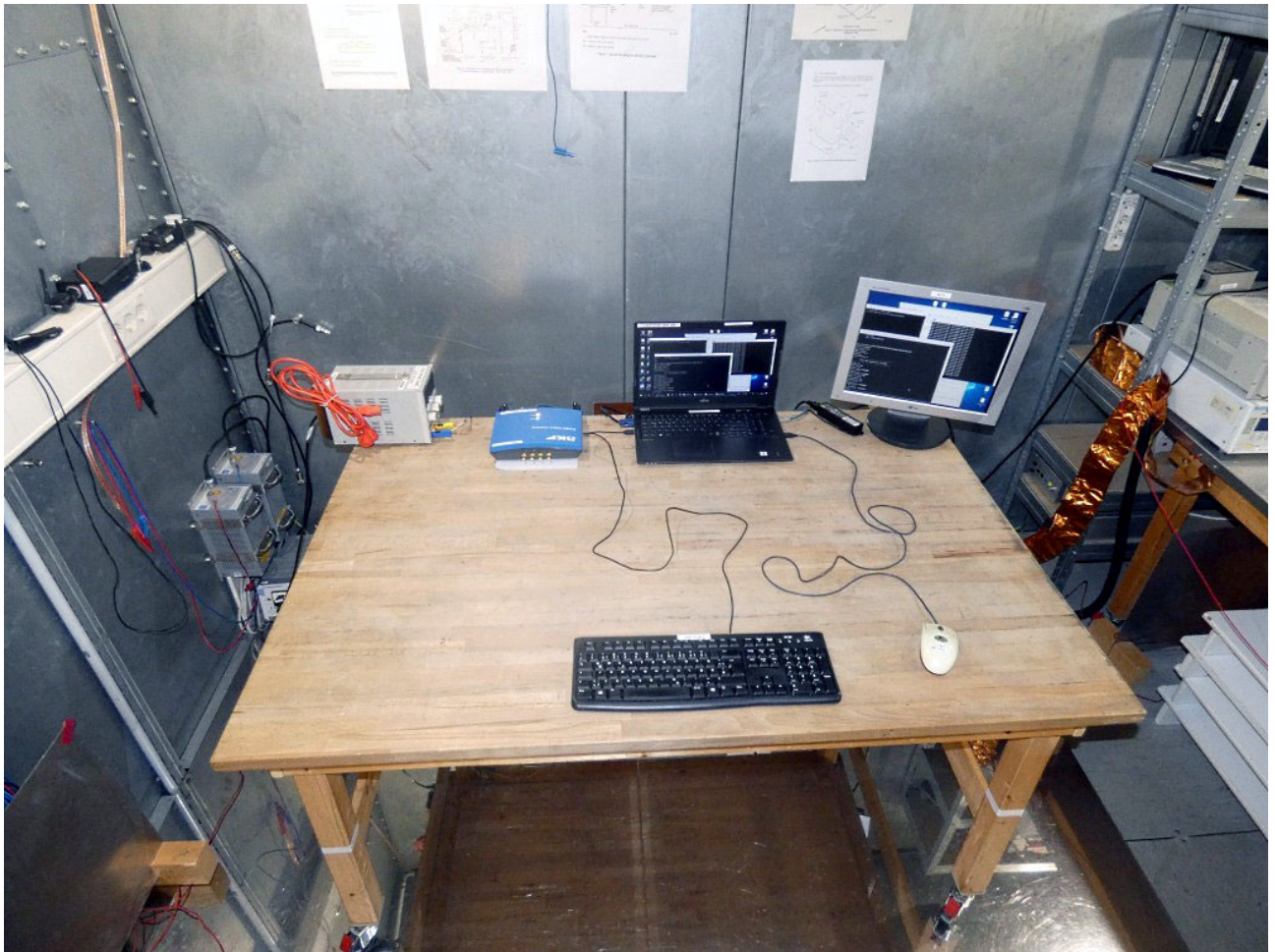
Photo 6: Test setup for conducted measurements (AC Port (power line), computer peripheral setup, EUT supplied by laboratory power supply, intentional / unintentional radiator §15, ANSI C63.4), complete test setup
