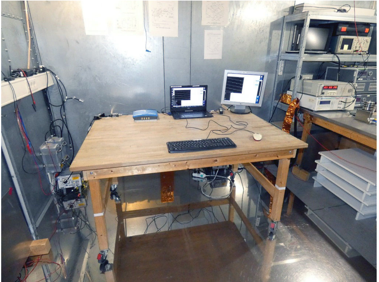
Photo 4: Test setup for conducted measurements (AC Port (power line), computer peripheral setup, EUT supplied by AC/DC adapter of PoE injector, intentional / unintentional radiator §15, ANSI C63.10/4), complete test setup
