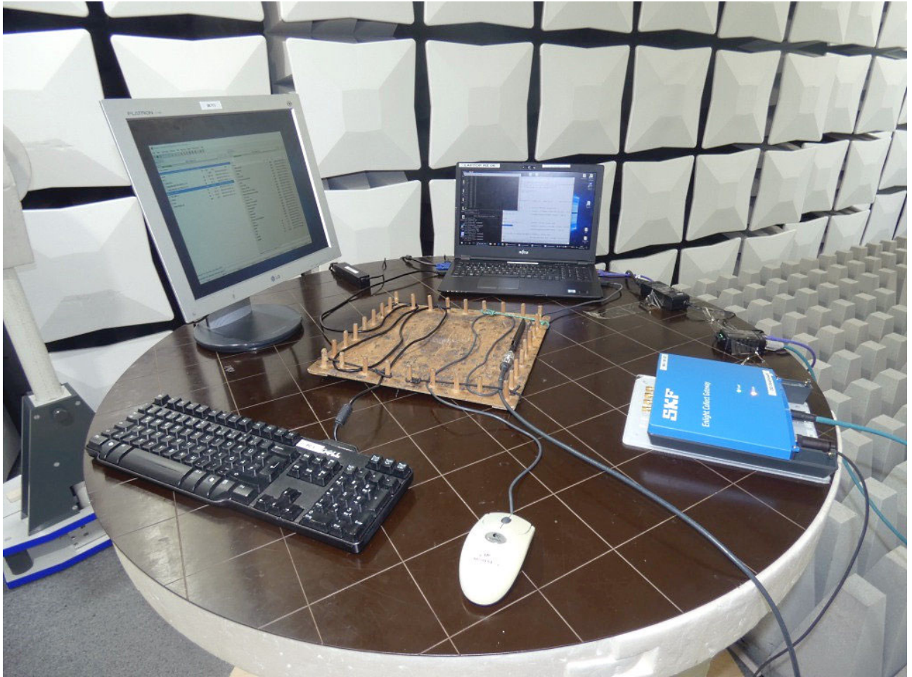
Photo 10: Test setup for radiated measurements (computer peripheral setup, EUT supplied by PoE, 18-26 GHz, unintentional radiator §15.109, ANSI C63.4)
