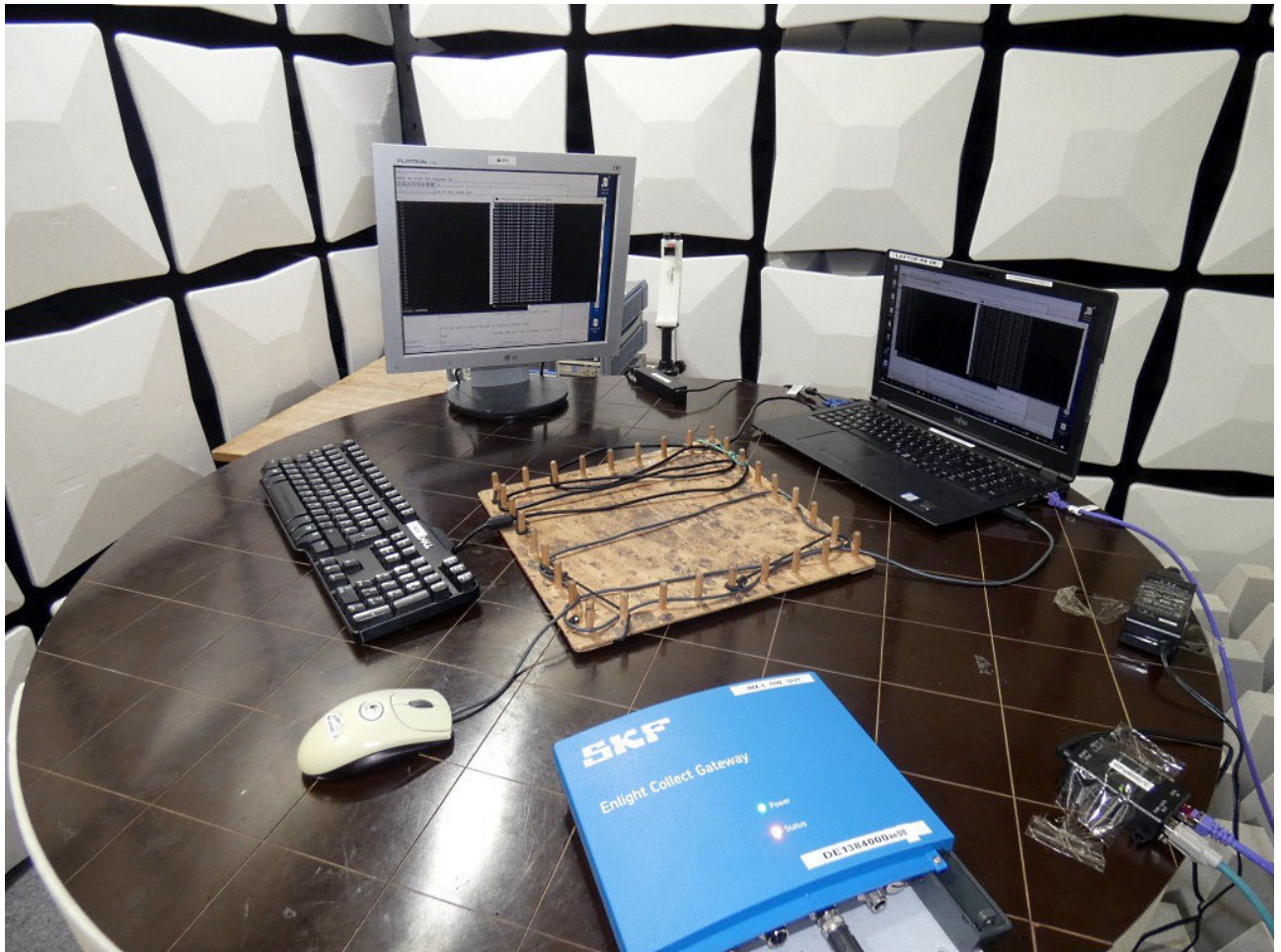
Photo 11: Test setup for radiated measurements (computer peripheral setup, EUT supplied by PoE, 26-40 GHz, unintentional radiator §15.109, ANSI C63.4)
