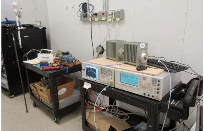
**RF RADIATED MEASUREMENT SETUP, 9 kHz - 30 MHz**
