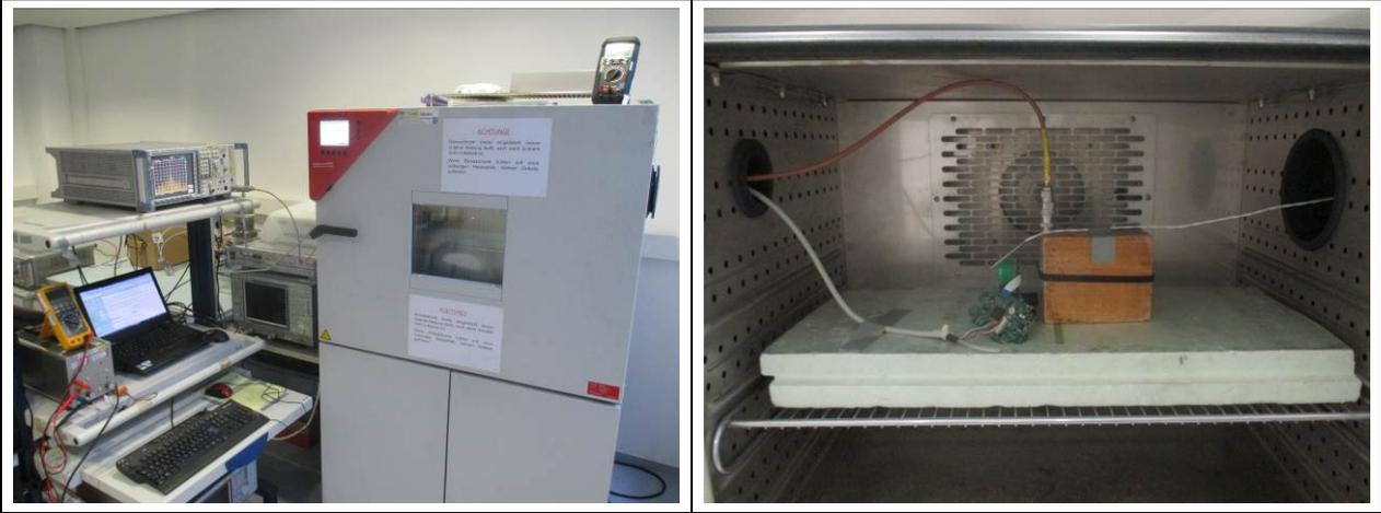
Figure 2: Test Setup Occupied Bandwidth – Configuration 2
