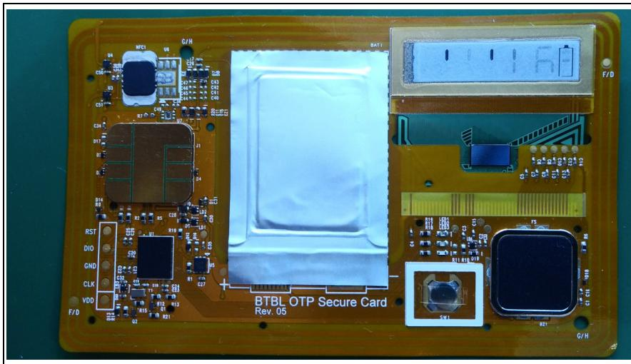
**Top view of Main PCB**
