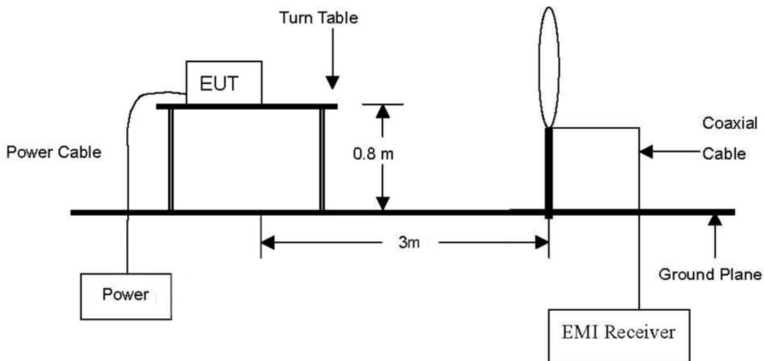
The diagram below shows the test setup that is utilized to make the measurements for emission from 30 MHz to 300 MHz Emissions.
