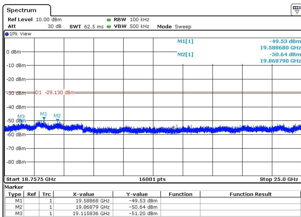
An additional consideration when performing conducted measurements of restricted-band emissions is that unwanted emissions radiating from the EUT cabinet, control circuits, power leads, or intermediate circuit elements will likely go undetected in a conducted measurement configuration. To address this concern, a radiated test shall be performed to ensure that emissions emanating from the EUT cabinet (rather than from the antenna port) also comply with the applicable limits.
