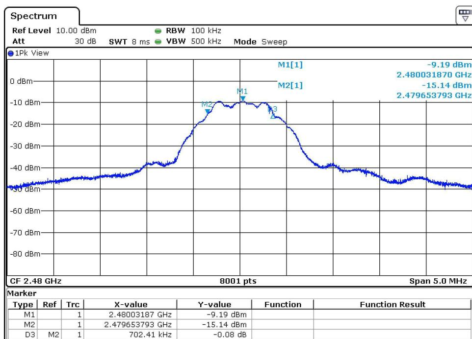
Conducted spurious emissions shall be measured for the transmit frequency, per 5.5 and 5.6, and at the maximum transmit powers.
