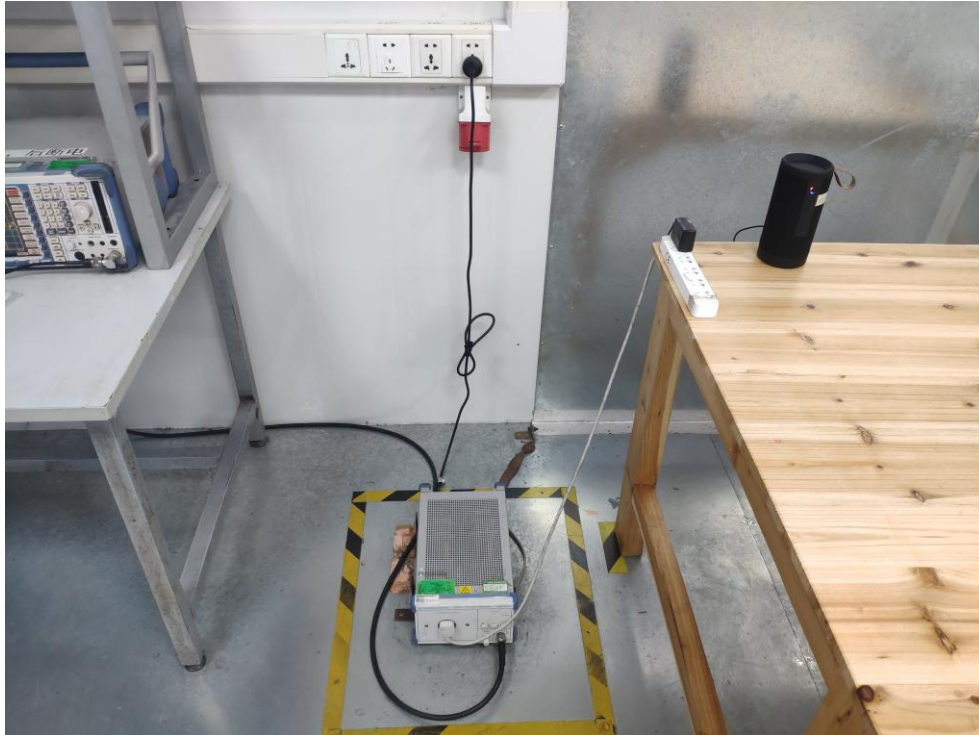
Photo of Conducted Emission Measurement
