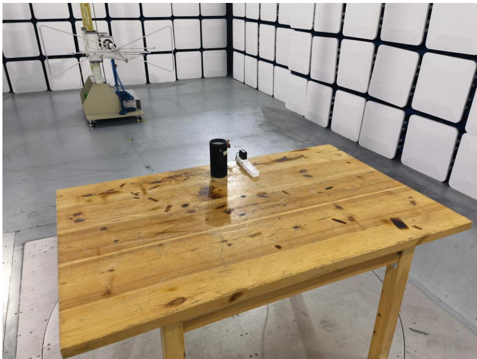
Photo of Radiation Emission Test
