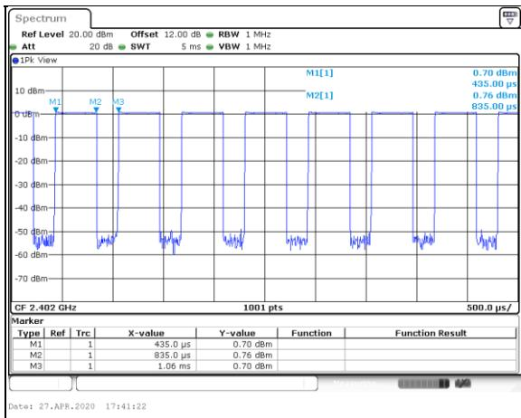
Note:  $T_{on} = \text{Mark2}-\text{Mark1}$ ,  $T_{on}+T_{off}=\text{Mark3}-\text{Mark1}$ .
