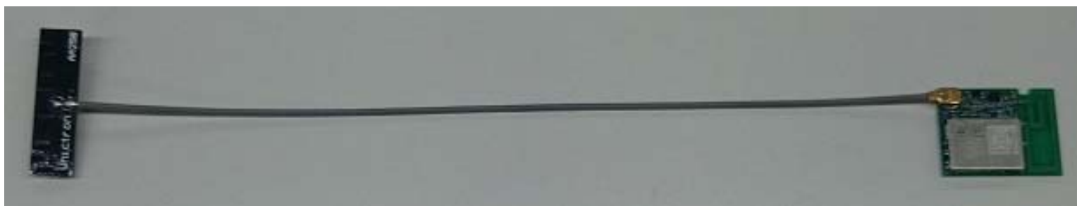
Top with external printed PCB antenna
