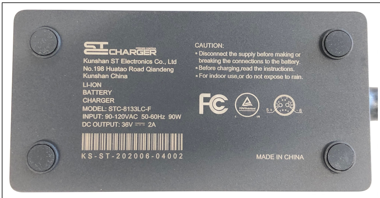
Figure 4-5: Copy of type plate of the charger STC-8133LC-F (Serial production)
