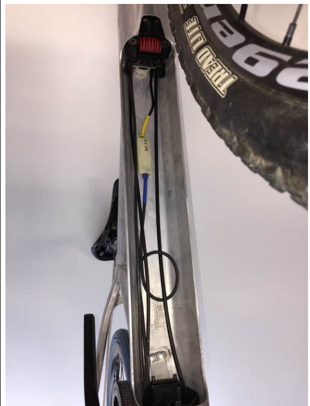
evaluation 12V Connector Box installed in the EPAC
