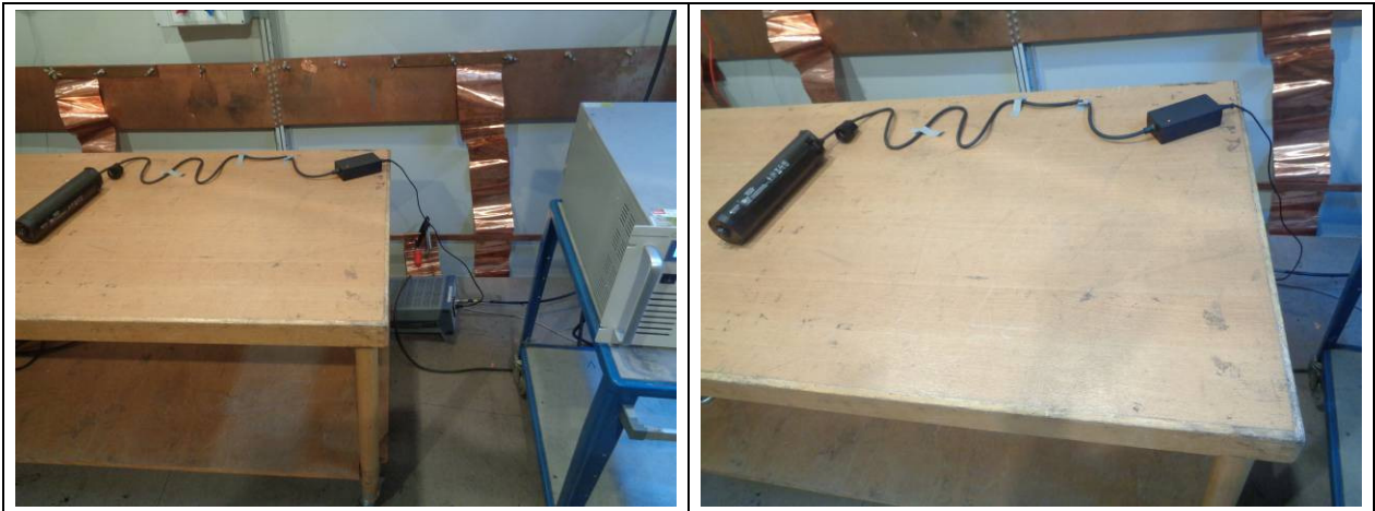
Figure 1: Test setup for conducted disturbance 150 kHz to 30 MHz – Configuration mode 2
