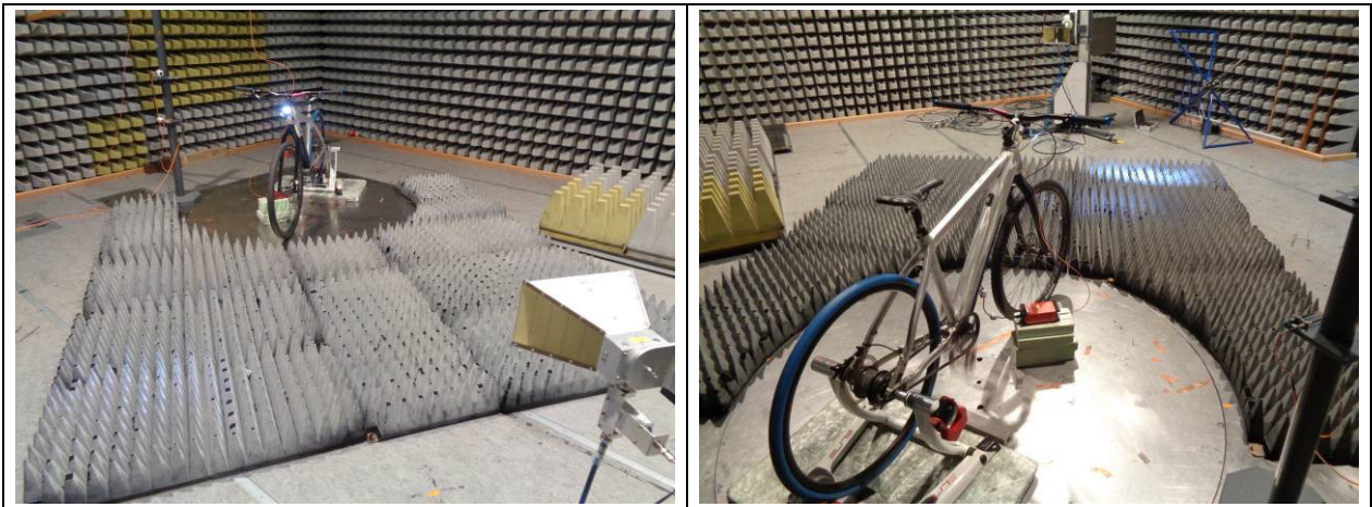
Figure 4: Test setup for radiated disturbances 1GHz to 18 GHz – Configuration mode 1
