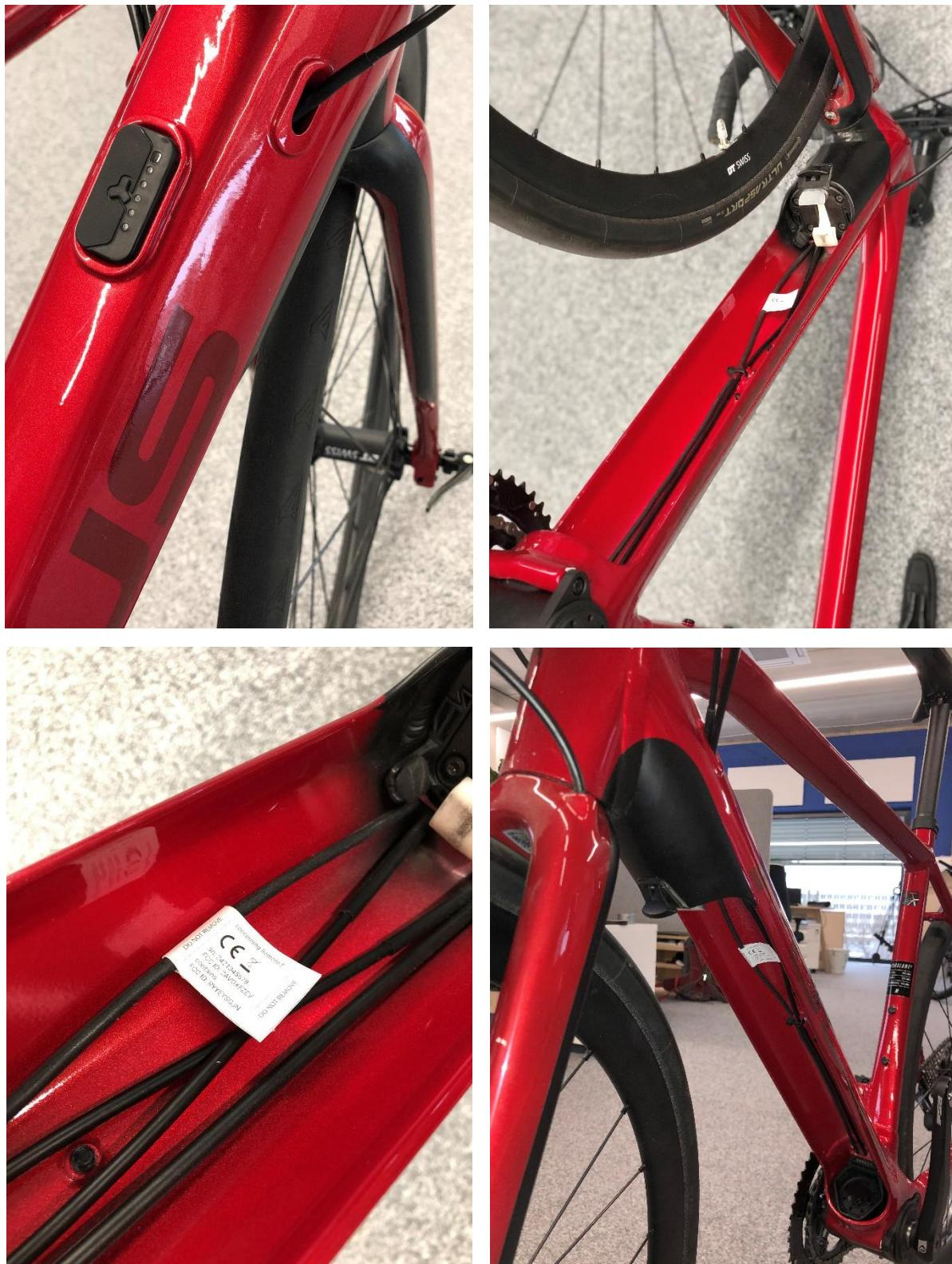
The remote in installed condition in the pedelec frame. The marking will be permanent visible to the end customer. Marked with permanent adhesive foil sticker – water resistand, temperature solid and printed on both sides.
