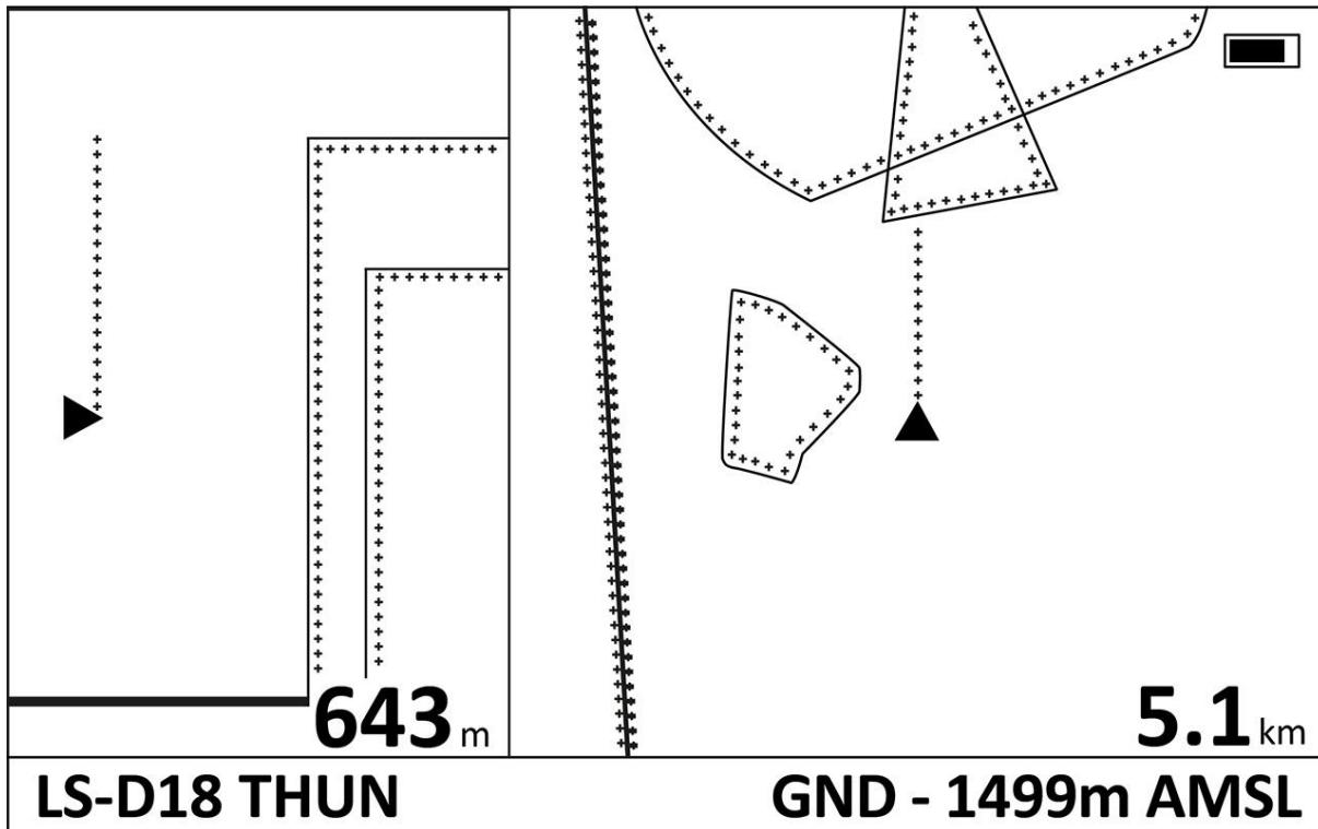
This is what the airspace screen from the Maxx II looks like when flying towards an airspace. On the left is the side view, on the right is the top view. The numbers indicate the vertical distance to the next airspace on the left, and the horizontal distance to the next airspace on the right.
