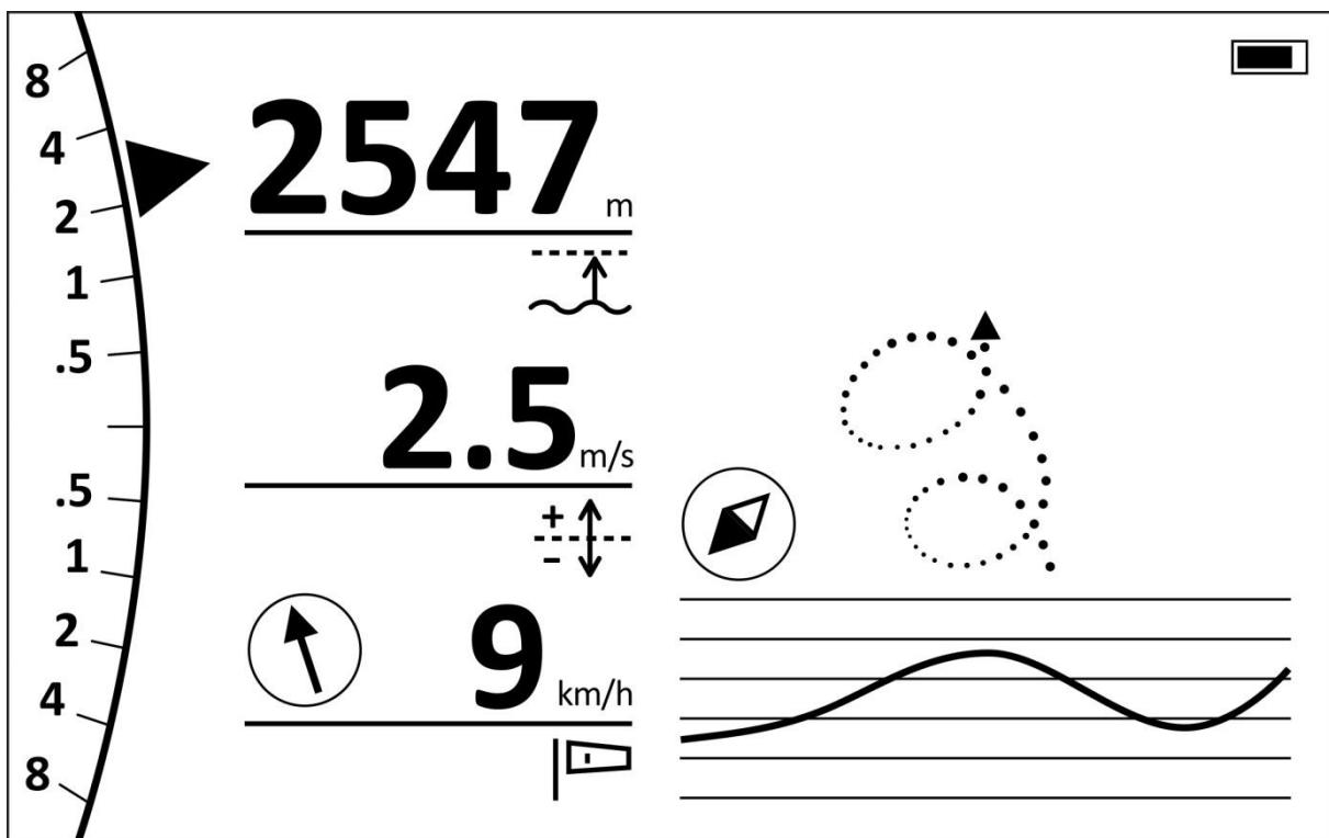
The analog vario display, as well as altitude, digital vario, wind and compass are displayed exactly the same as on the standard screen.
