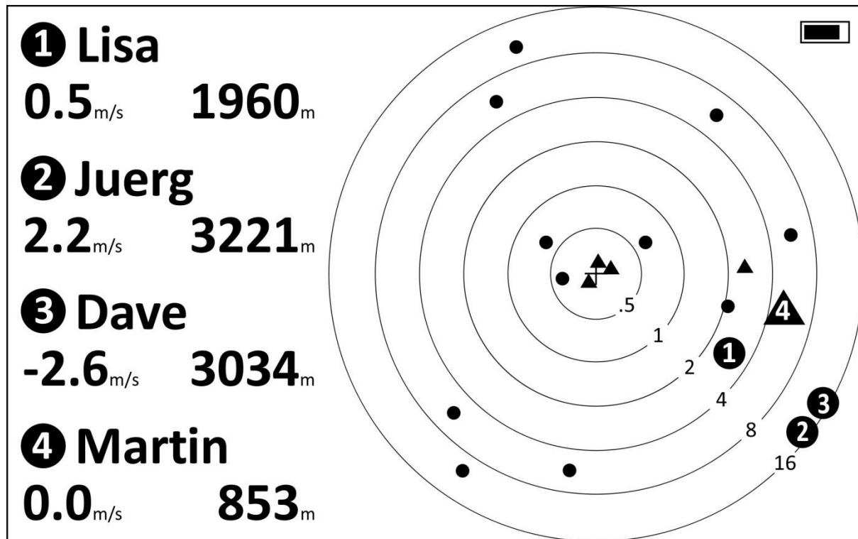
On the Buddy Screen you can see all paraglider and hang glider pilots who fly with a FLARM / FANET device and have been received by the XC Tracer Maxx II in the last 5 minutes. Your position is in the middle of the circles, and from one circle to the next the distance (in kms) doubles.
