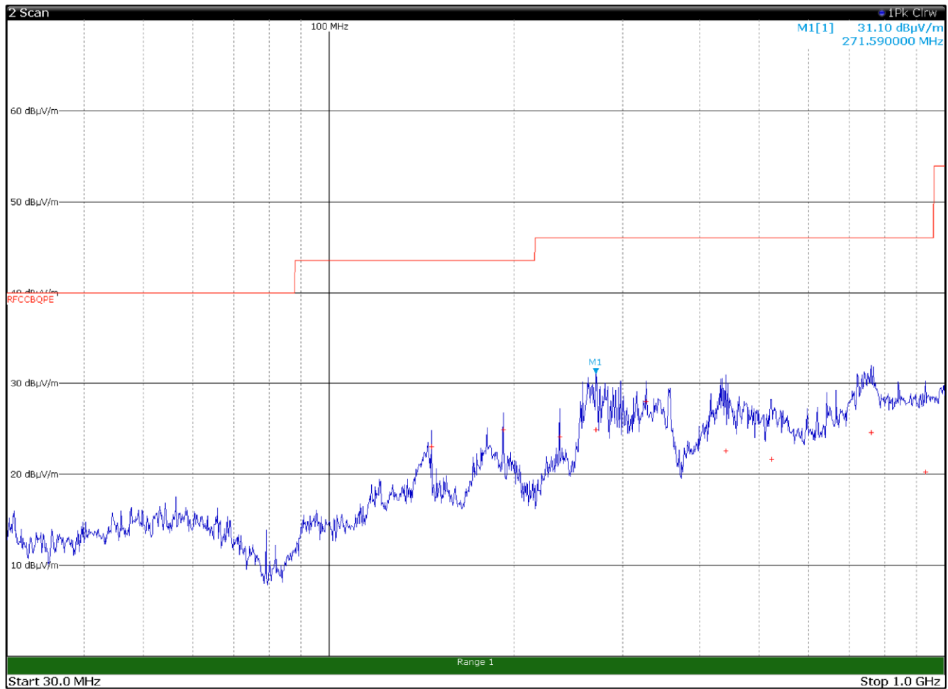
Figure 8.4-11: Radiated spurious emissions for the WIRELESS REM PROBE BLU, mid channel with antenna in horizontal polarization
