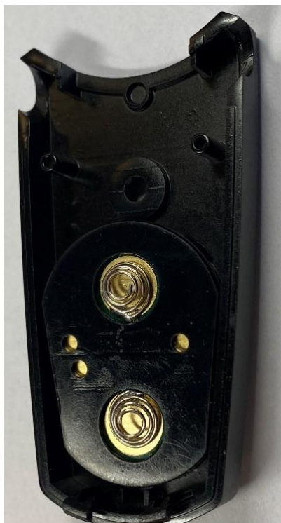
Wireless probe back shell with board protection
