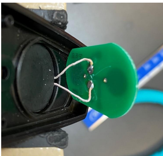
Wireless probe back shell with RE1-EL006 board and coil
