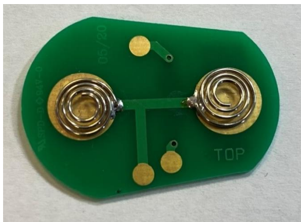
RE1-EL006 board – top view with battery pins soldered
