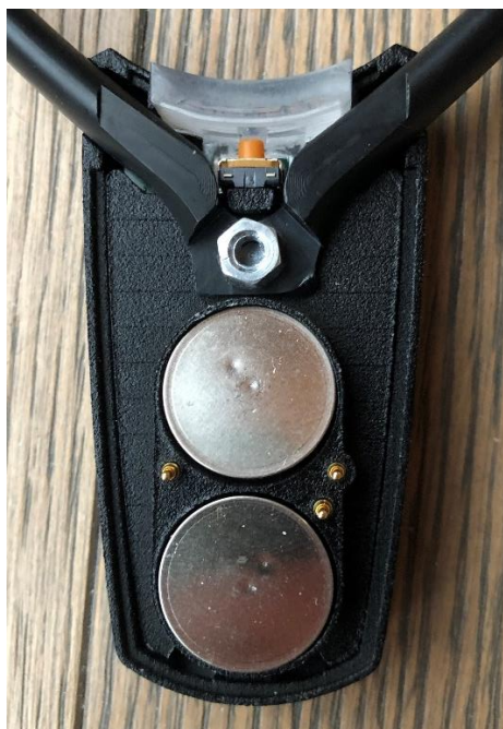
Wireless probe front shell with batteries
