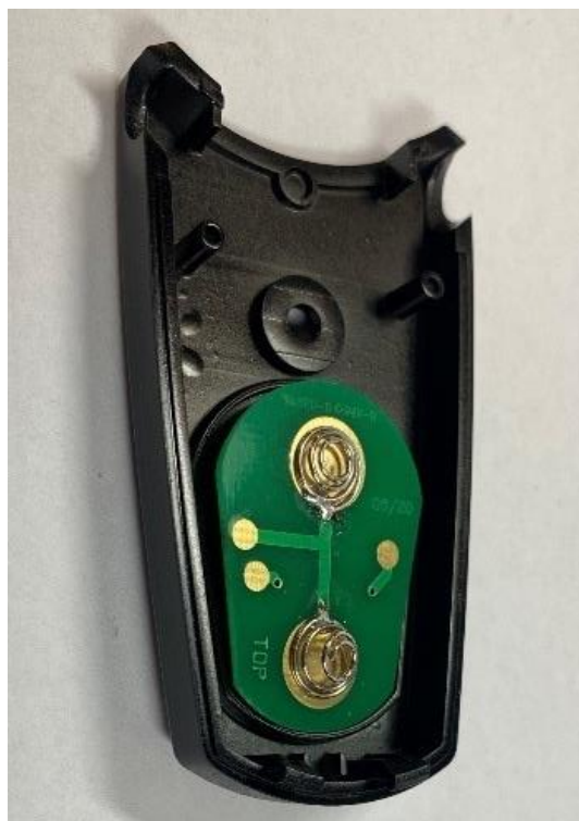
Wireless probe back shell without protection
