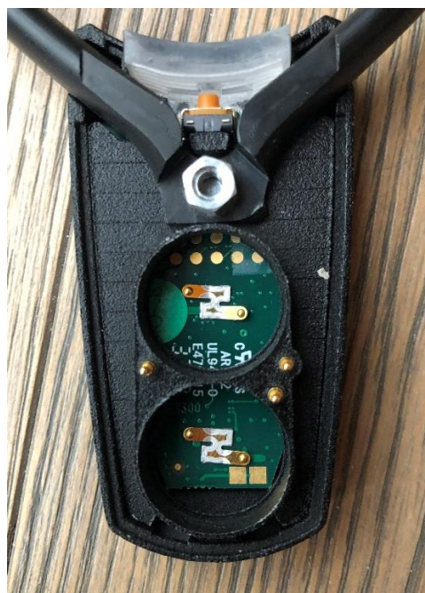
Wireless probe front shell without batteries
