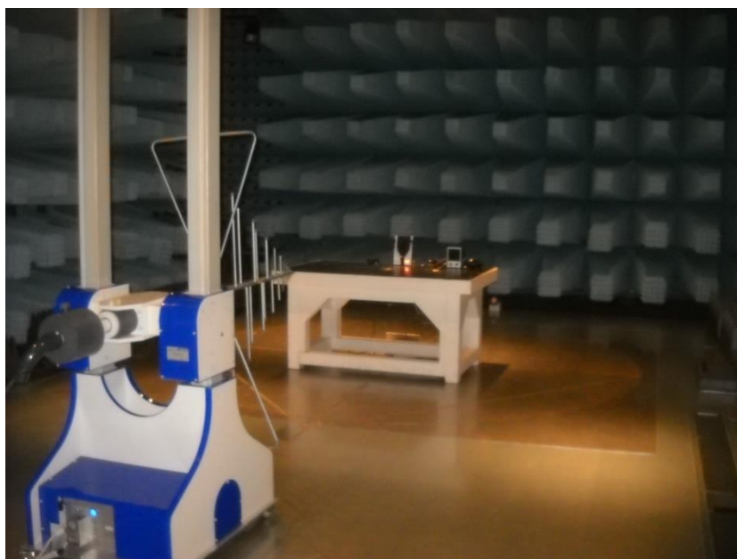
Set-up for radiated emission test below 1 GHz (base unit)
