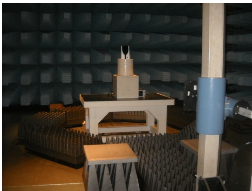
Set-up for radiated emission test above 1 GHz (base unit)
