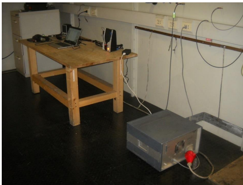
Set-up for conducted emission test
