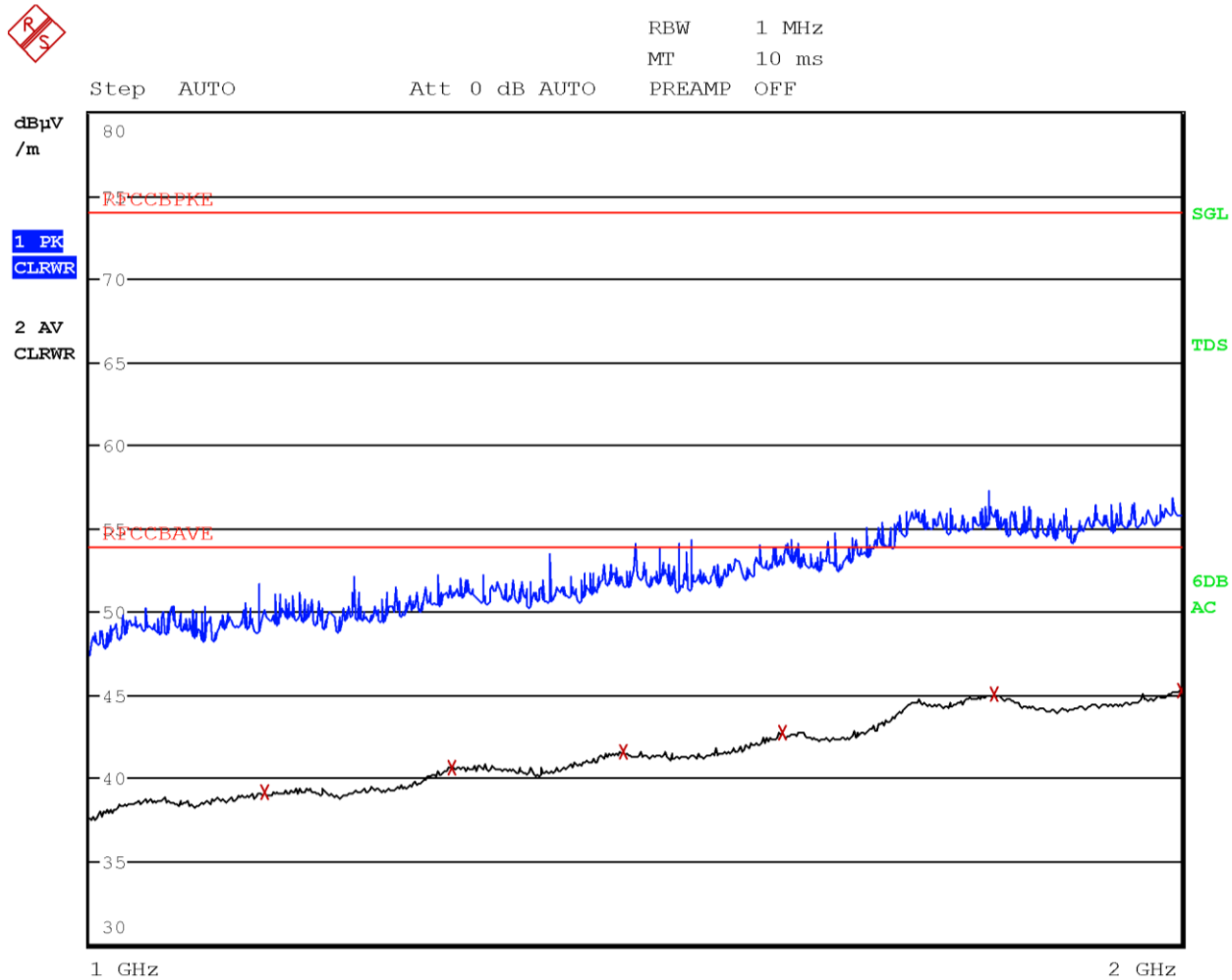
Figure 8.3-5: Radiated field strength measurement results for frequency above 1000 MHz – Antenna in vertical polarization
