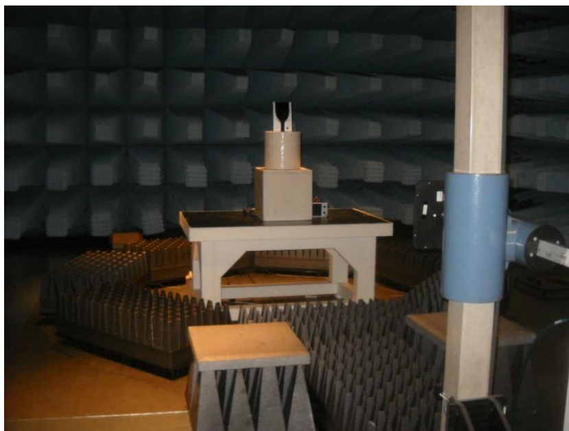
Set-up for radiated emission test above 1 GHz (REM probe)
