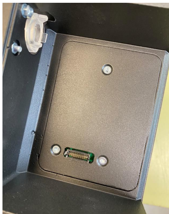
RE1-EL009 board bottom part assembly
