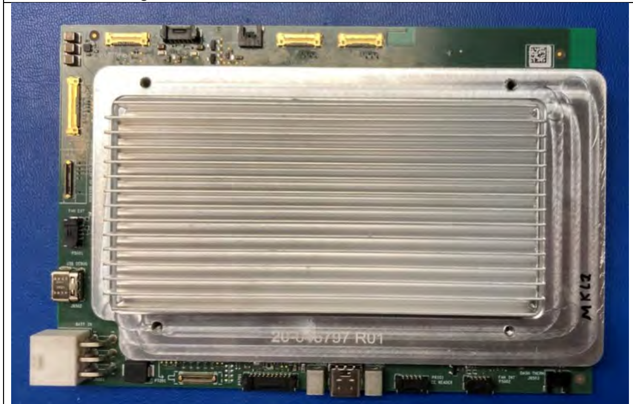
Dashboard's Main Logic Board with WiFi
