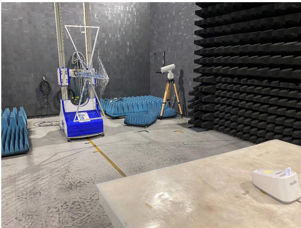
Test set up radiated emission 30 MHz – 1 GHz
