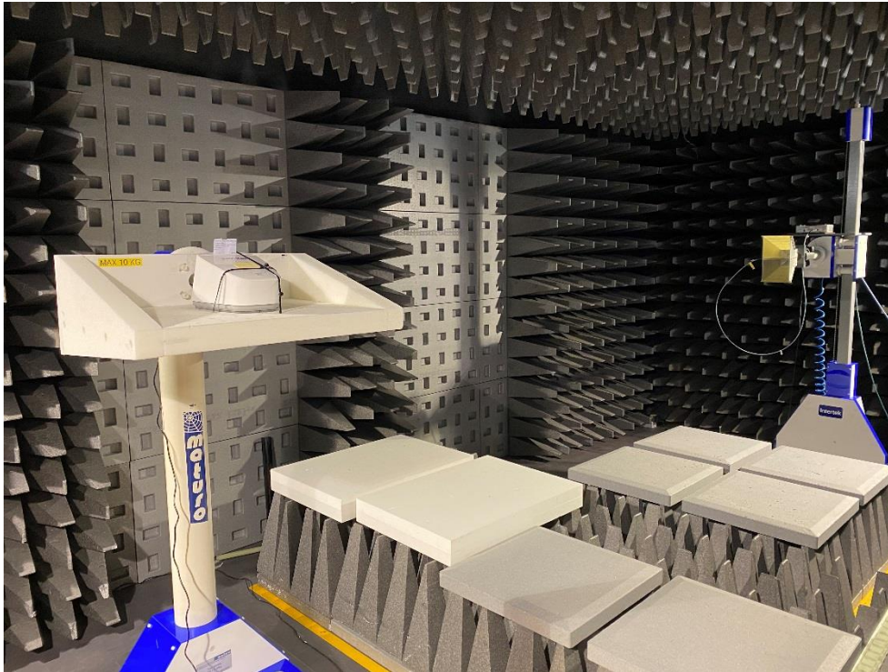
Test set up radiated emission above 1 GHz
