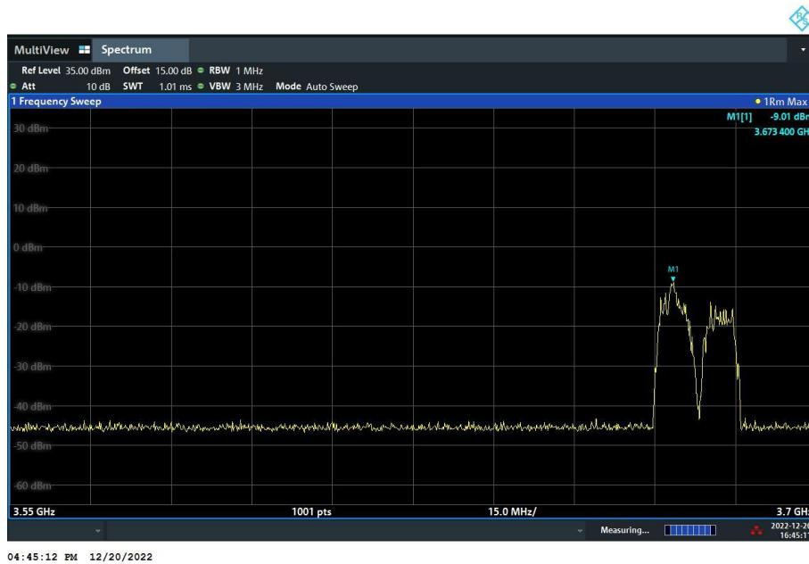
**[Step 8.a.]** After changing the frequency and power level, The module (EUT) discontinues operations, change frequencies, or change its operational power level within 10 seconds of receiving instructions from its associated CBSD. Test result is PASS.
