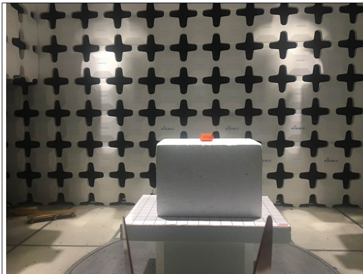
Radiated Emission Test above 1GHz Front View
